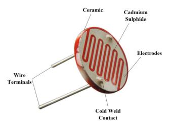
Figure 8. Light Dependent Resistor.
