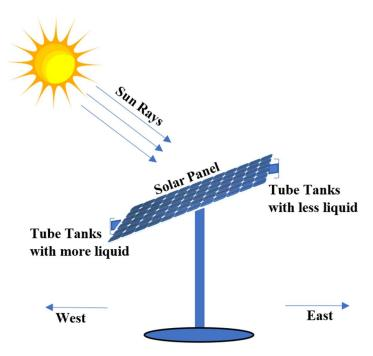
Figure 7. Passive Tracking System.
