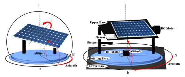
Figure 4. Various Dual-axis Solar Tracking Systems. (a) TTDAT; (b) AADAT.
