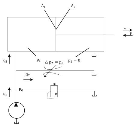
Figure 10. Schematic diagram of the throttle speed control loop.
