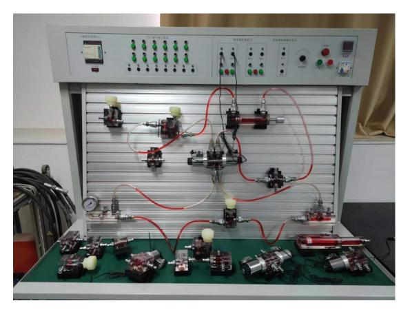
Figure 5. Traditional "Hydraulic Transmission" course experimental platform.
