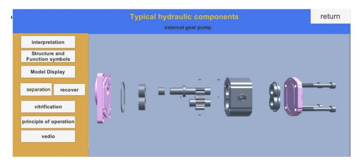
Figure 9. Automatic disassembly and assembly of the external gear pump.
