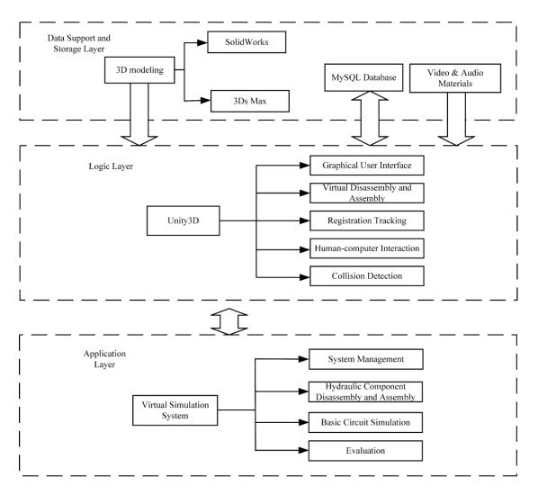
Figure 4. Development framework diagram of the hydraulic transmission teaching system.
