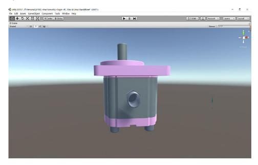
Figure 6. Three-dimensional (3D) model of an external gear pump.
