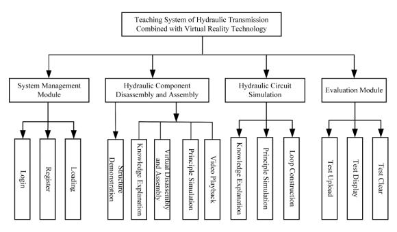
Figure 3. The functional structure of the hydraulic transmission teaching system.
