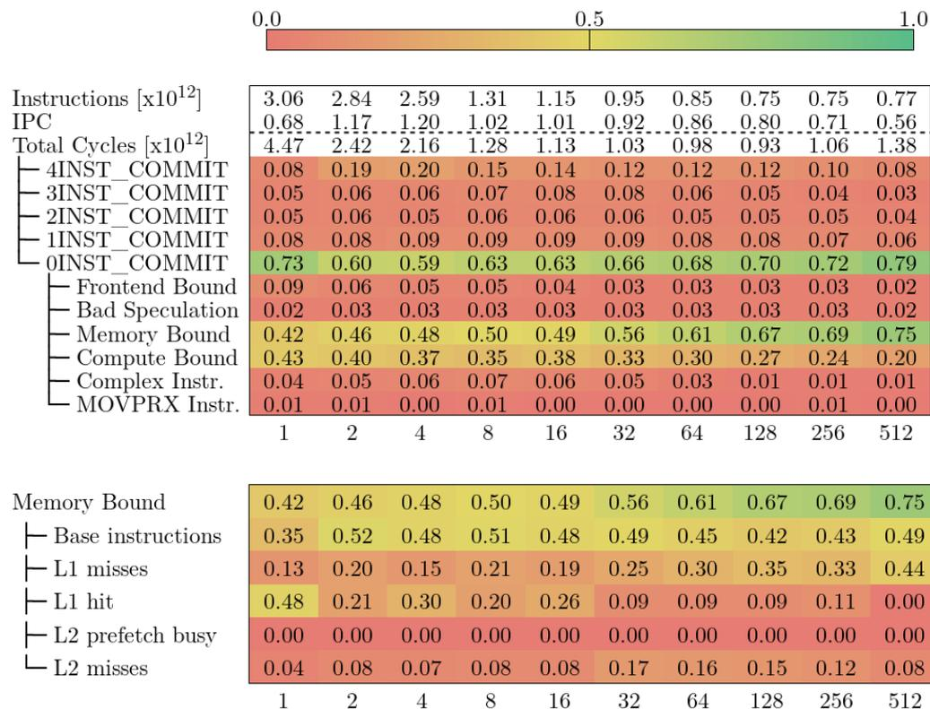
Figure 12. Top-Down model for Alya in CTE-Arm.
