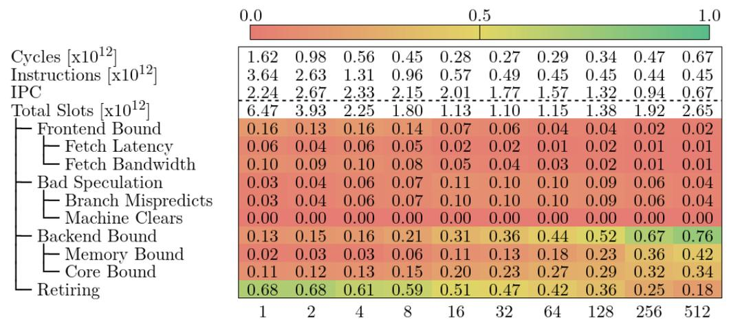
Figure 9. Top-Down model for Alya in MareNostrum 4.
