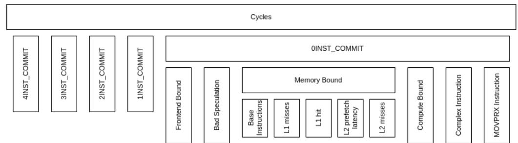
**Figure 3.** Top-Down model hierarchy in CTE-Arm.
