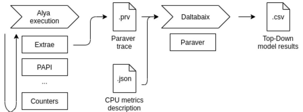
Figure 8. Workflow from application execution to model results.
