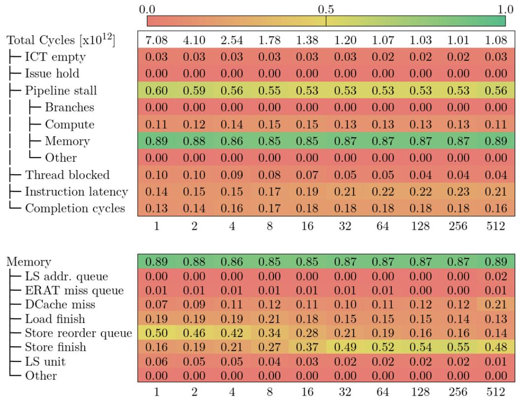
Figure 13. Top-Down model for Alya in CTE-Power.
