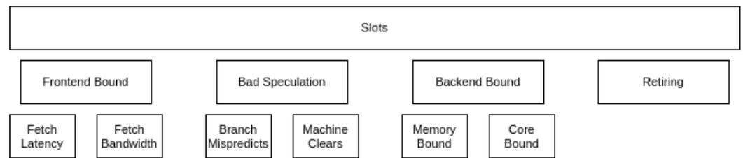
**Figure 1.** Top-Down model hierarchy in MareNostrum 4.
