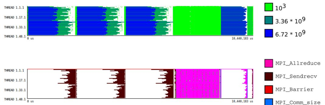
**Figure 7.** Paraver timeline examples. **Top:** quantitative representation of number of instructions. **Bottom:** MPI primitive calls.
