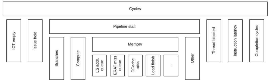
Figure 4. Top-Down model hierarchy in CTE-Power.
