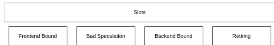
**Figure 2.** Top-Down model hierarchy in CTE-AMD.
