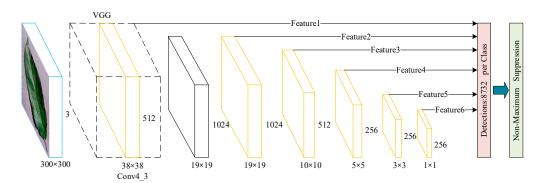
Figure 1. SSD backbone network structure.
