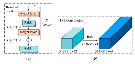
**Figure 4.** (a) Residual network module and (b)  $1 \times 1$  convolution.
