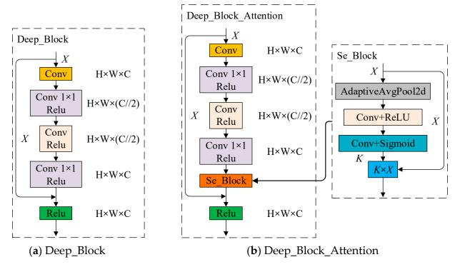
**Figure 5.** Enriched feature extraction module ((**a**) Deep\_Block, a feature extraction module combining residual network and  $1 \times 1$  convolution; (**b**) Deep\_Block\_Attention, a feature extraction module adding an attention mechanism to (**a**)).
