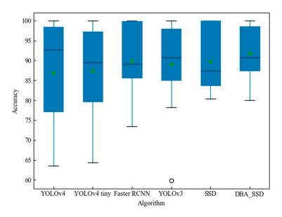
**Figure 15.** Box plot of AP statistics under target detection algorithm.
