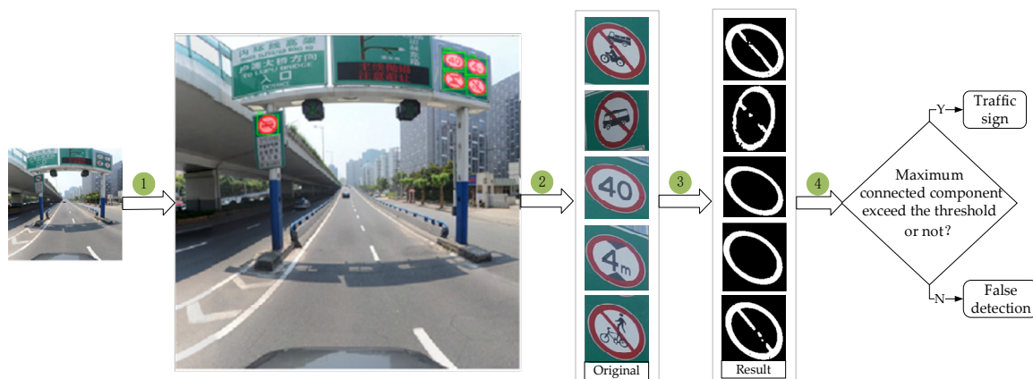
Figure 1. Flow chart of lightweight SSD-based traffic sign detection.
