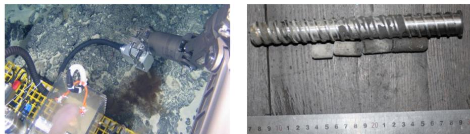
Figure 15. Deep-sea drilling operation and core collected from a cobalt crust on the seafloor.
