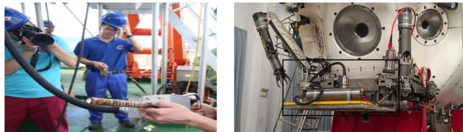
Figure 14. The drilling apparatus on the Jiaolong submersible.
