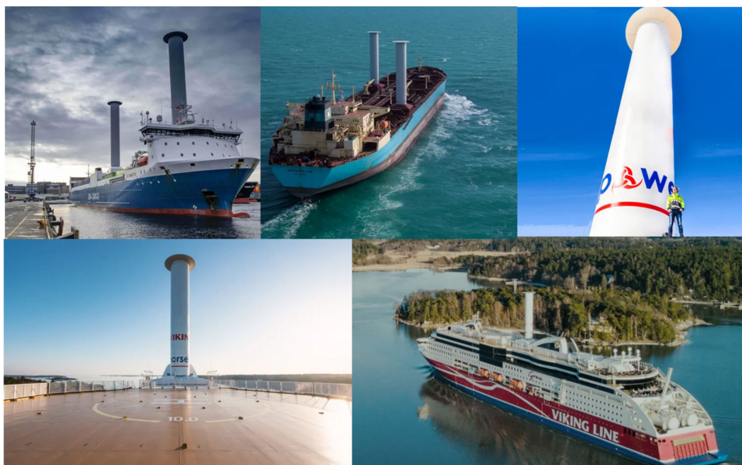
Figure 7. Examples of vessels with Flettner rotors installed, different vessel types: RoRo vessel, tanker and ferry, Image courtesy: Norsepower Oy Ltd.
