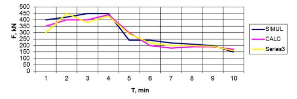
**Figure 11.** Tug's towage forces during ship's unmooring and departure operations, obtained by calculation (CALC) and simulation (SIMUL) during real operation with similar vessel under hydrometeorological conditions (Series3) (wind N—14 m/s).
