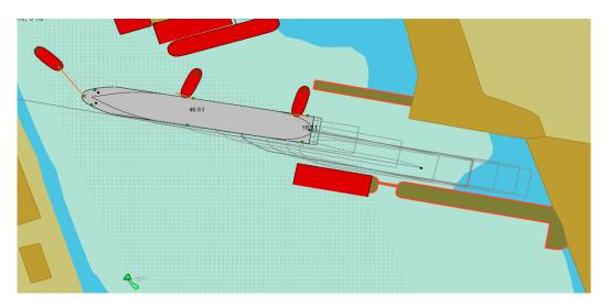
**Figure 18.** Ship (L = 238 m) moving off the berth with south direction wind of 14 m/s, and three tugs were used located as follows: the first in towage position and the second and third in push/pull position, all three tugs acting.
