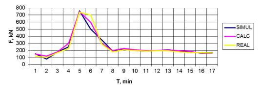
**Figure 15.** Tug towage line tension and pull/push forces during ship's unmooring, manoeuvring and departure operations, obtained by calculation (CALC) and simulation (SIMUL) during real ship operation with similar vessel under hydro meteorological conditions (REAL) (wind W—14 m/s).
