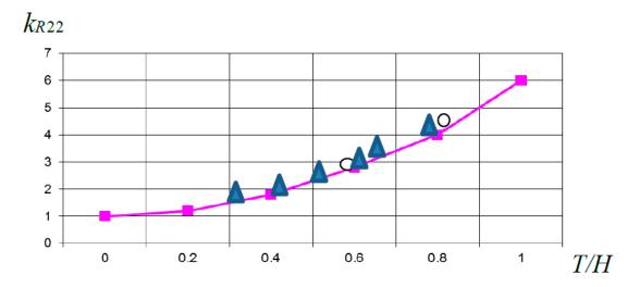
**Figure 3.** Ship's additional coefficient of resistance  $k_{R22}$ , depending on ship's draft and depth T/H (calculation and experimental "o" for the tanker L = 250 m and ("  $\blacktriangle$  ") for the container vessel L = 365 m results).
