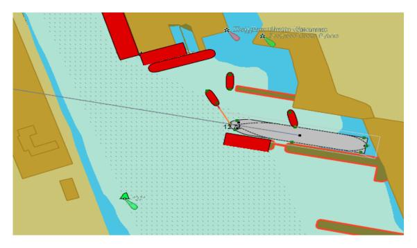
**Figure 16.** Ship (L = 238 m) departure from berth in the case of south direction wind—14 m/s and tugs location (three tugs were used: the first in towage position, the second in push/pull position and the third in stand-by position).
