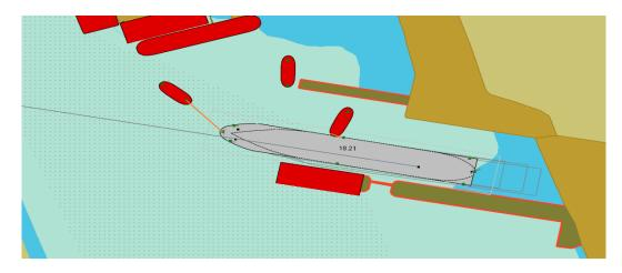
**Figure 17.** Ship (L = 238 m) moving off the berth with south direction wind of 14 m/s, and three tugs were used, located as follows: the first in towage position, the second in push/pull position and the third in stand-by position.
