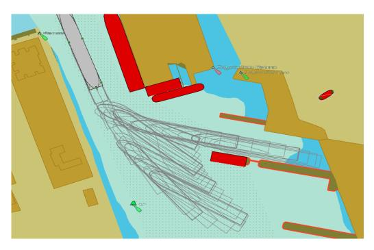
**Figure 14.** Ship's (L = 238 m) departure trajectory in the case of wind W—14 m/s.
