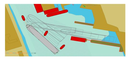
**Figure 19.** Ship (L = 238 m) moving off the berth with south direction wind of 14 m/s, and three tugs were used located as follows: the first in towage position, and the second and third in push/pull position and ending with push/pull operation.
