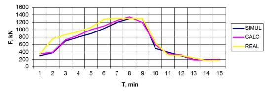
**Figure 21.** Tug towage line tension and pull/push forces during ship's unmooring, manoeuvring and departure operations, obtained by calculation (CALC) and simulation (SIMUL) during real operation with similar vessel under hydrometeorological conditions (REAL) (wind S—14 m/s).
