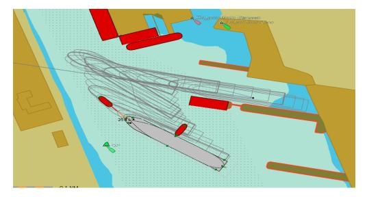
Figure 13. Ship's departure trajectory with wind W—14 m/s until tug No 2 stopped push/pull operation.
