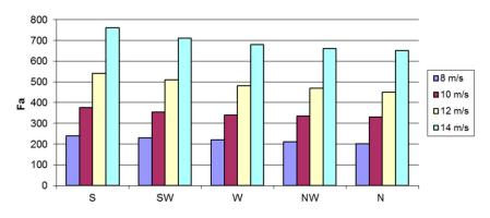
Figure 9. Wind forces on ship (L = 238 m) depend on wind direction and speed.
