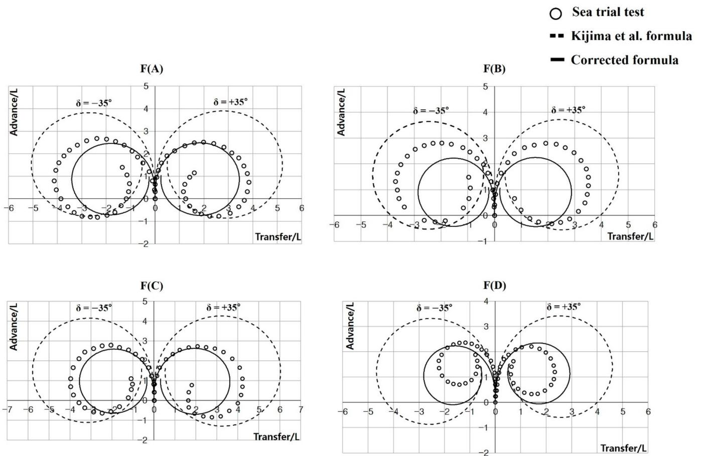
**Figure 5.** Comparison of turning movement test results in model fishing vessels.
