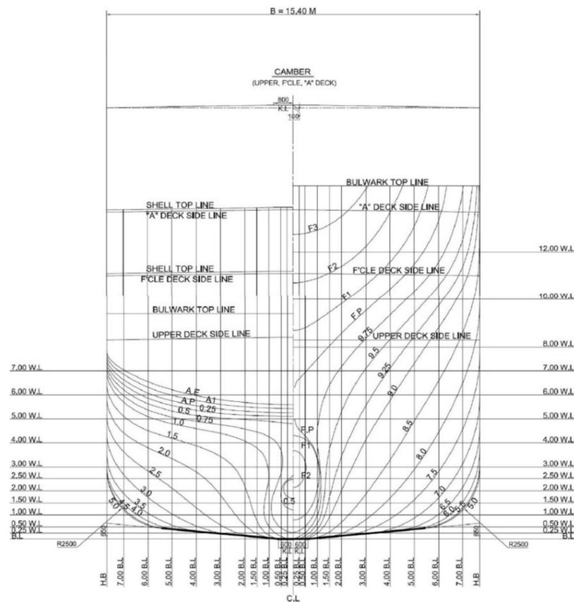
**Figure 6.** Body plan of target fishing vessel.
