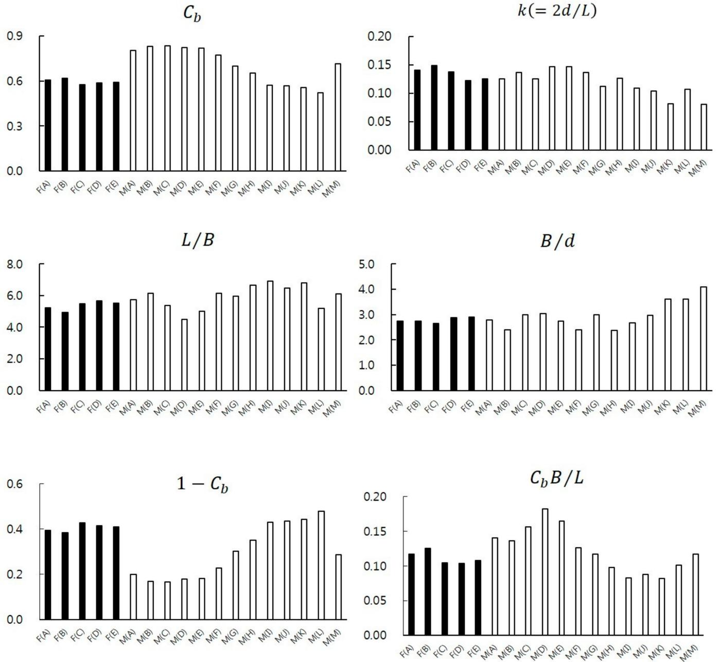
Figure 2. Hull shape parameters of 18 ships.
