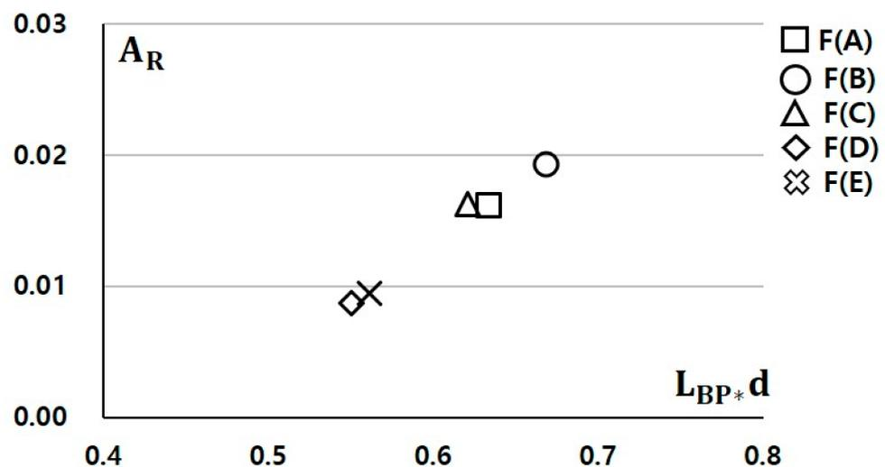
**Figure 8.** Rudder area ratio of model fishing trawlers.
