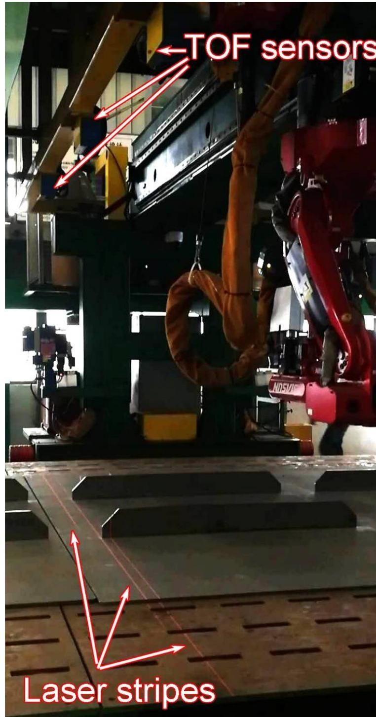
**Figure 3.** TOF sensors scan over small assemblies.
