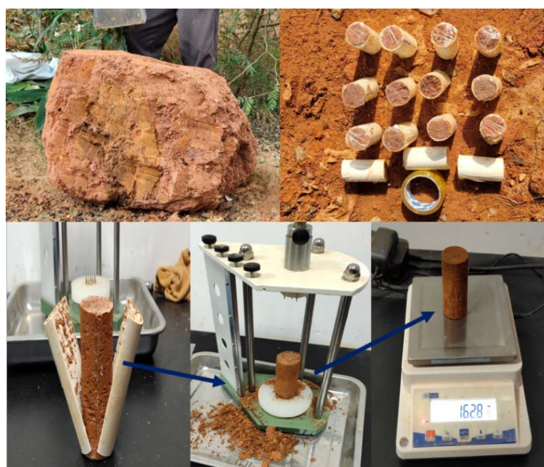
Figure 3. Trimming of the intact samples.
