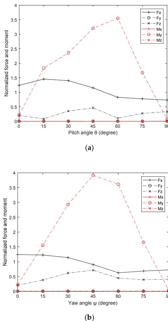
**Figure 14.** Normalized forces and moments on the cuboid payload versus a single posture angle when the roll angle  $\phi = 90^\circ$ . (a) the pitch angle  $\theta$ ; (b) the yaw angle  $\psi$ .
