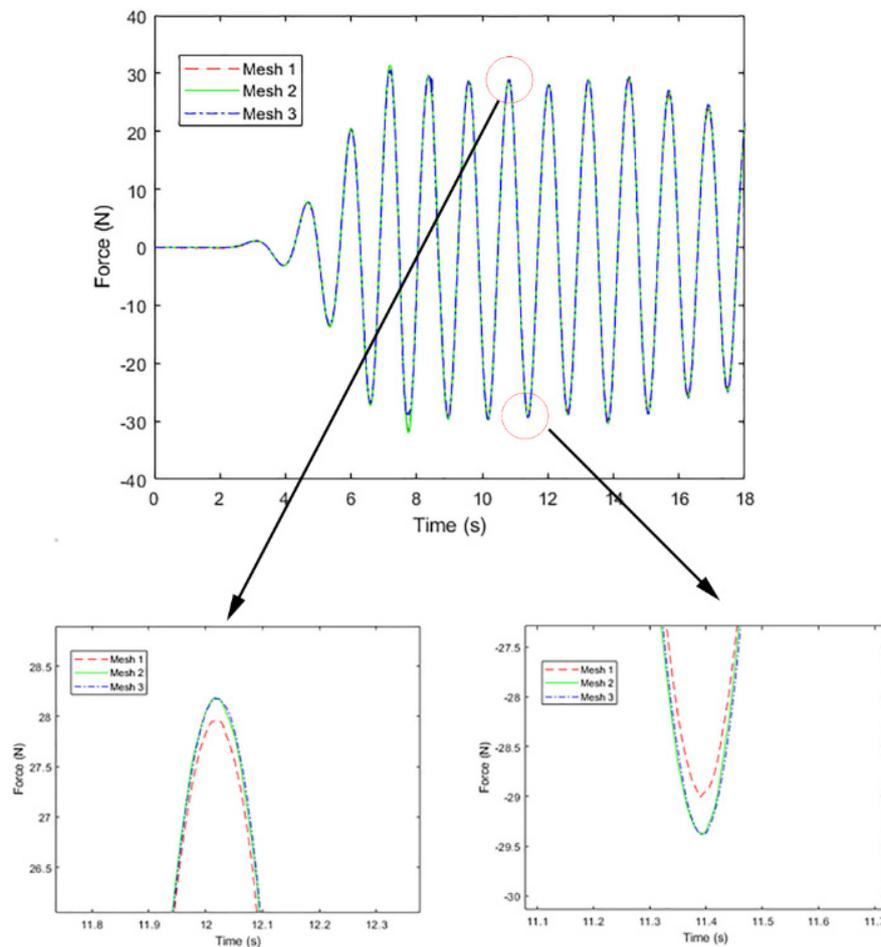
**Figure 6.** Time history of horizontal force  $F_x$  on the cylinder payload with three different mesh schemes for regular wave R1.
