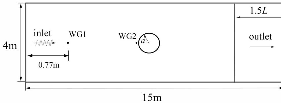
Figure 3. Layout of the numerical wave tank.
