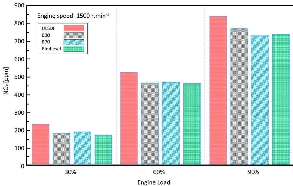
Figure 9. The dependence of testing fuels on the NO<sub>x</sub> emissions (1500 rpm).
