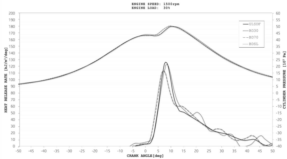
Figure 5. The dependence of fuels on the heat release rate and cylinder pressure (1500 rpm/30%).
