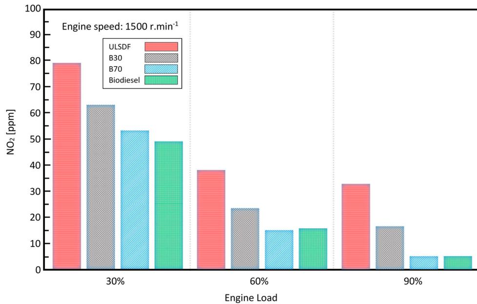
**Figure 11.** The dependence of testing fuels on the NO<sub>2</sub> emissions (1500 rpm).
