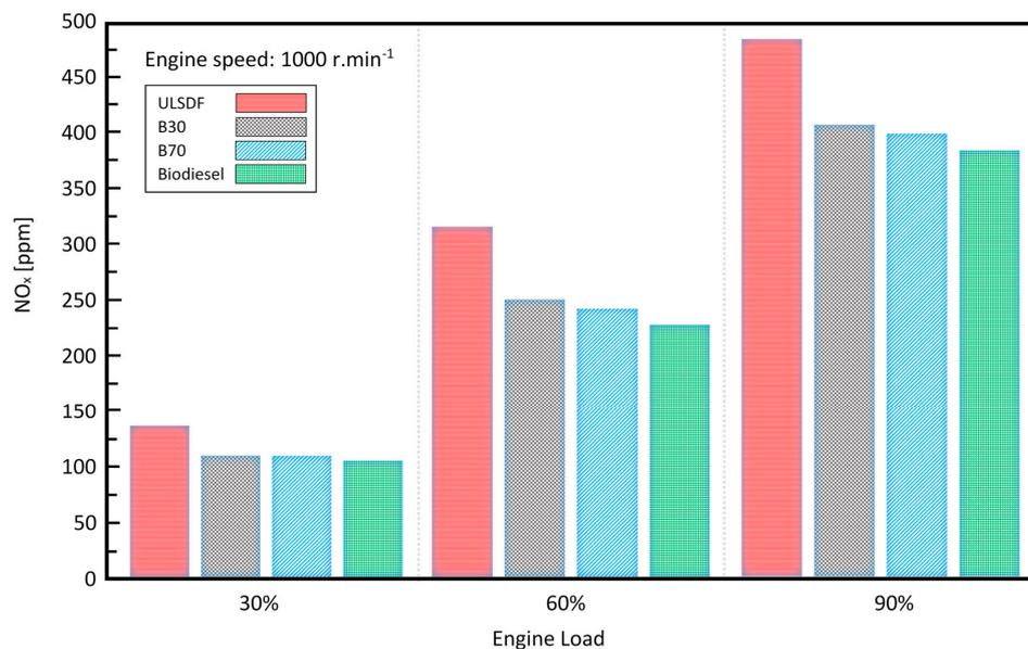
Figure 8. The dependence of testing fuels on the NO<sub>x</sub> emissions (1000 rpm).
