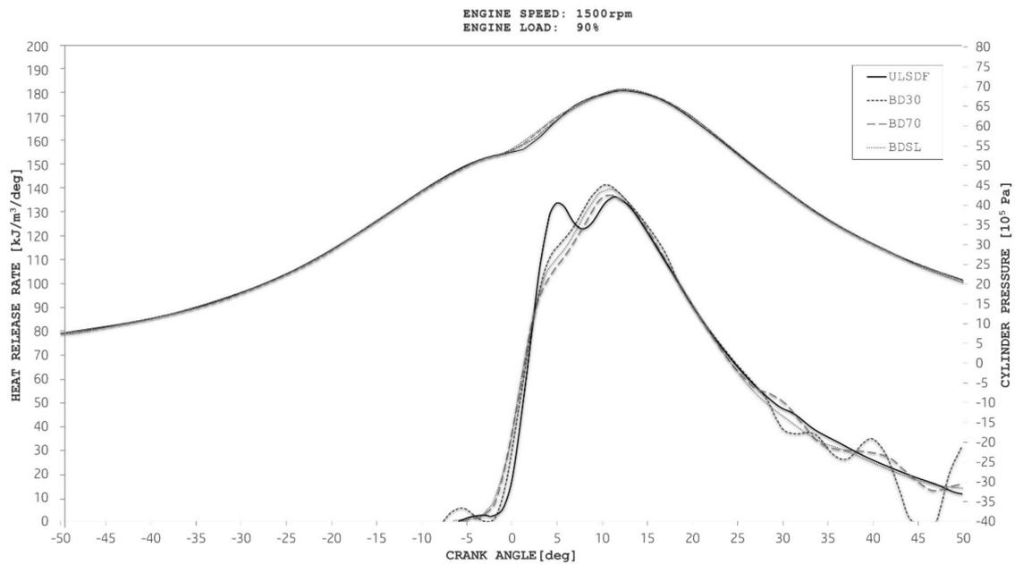
Figure 7. The dependence of fuels on the heat release rate and cylinder pressure (1500 rpm/90%).
