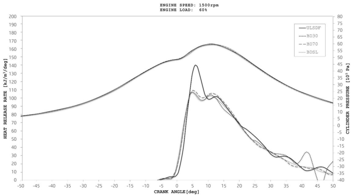
Figure 6. The dependence of fuels on the heat release rate and cylinder pressure (1500 rpm/60%).
