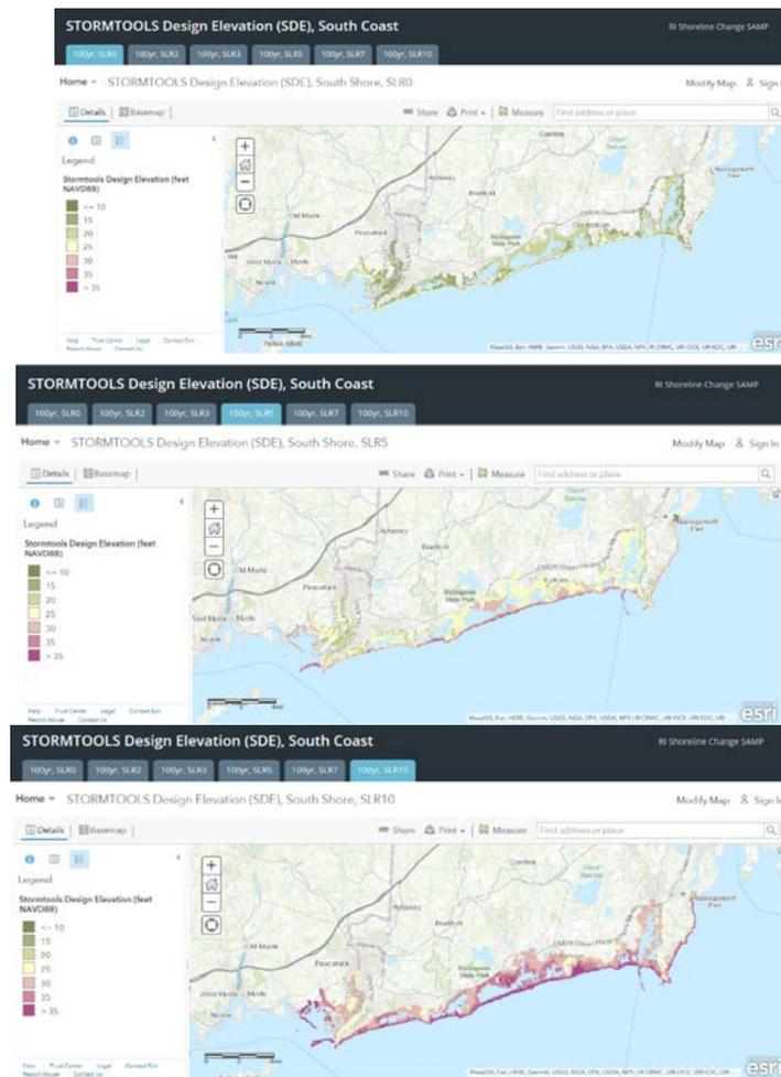
**Figure 6.** Impact of SLR on Narragansett Bay SDE maps, cases shown are 0, 5 ft, and 10 ft (0, 1.5, and 3 m) (upper, middle, and lower panels, respectively, note highlighted tab) SLR. (Note that the background map in these figures used the topographic map shown earlier. Background maps were user selected.).
