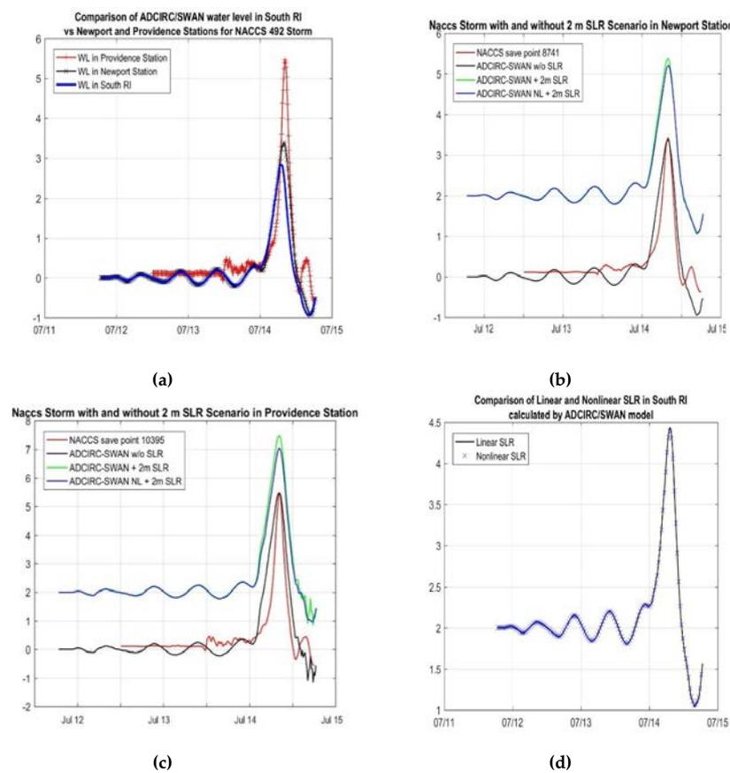
**Figure 3.** (a) Water level vs. time for NACCS storm #492 at Providence, Newport, and Charlestown, RI; (b) ADCIRC-SWAN-predicted water level vs. time for NACCS storm #492 at Newport without sea level rise (SLR), with 6.6 ft (2 m) of SLR simply added on, and with 2-m SLR added to the initial bathymetry and simulations run with the full model, (c) same as in (b) but at the Providence station; and (d) results of linear (superposition) and nonlinear simulation at Charlestown.
