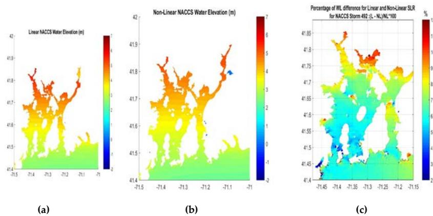
**Figure 4.** Peak water level for NACCS storm #492 for Narragansett Bay for (a) linear superposition method, (b) full nonlinear simulation results, and (c) percent (%) difference between the two for 6.6-ft (2-m) SLR.
