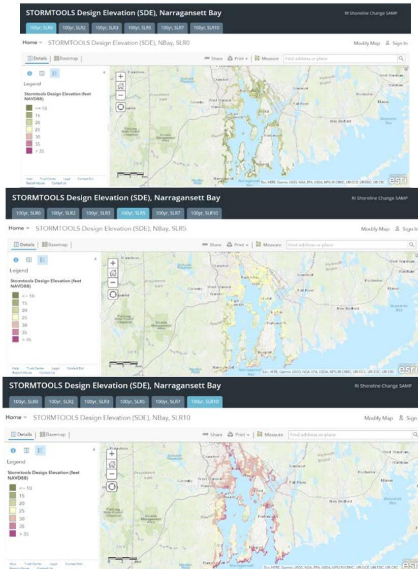
**Figure 11.** Impact of SLR on Narragansett Bay SDE maps, cases shown are 0, 5 ft (1.52 m), and 10 ft (3.05 m) SLR (upper, middle, and lower panel, respectively).
