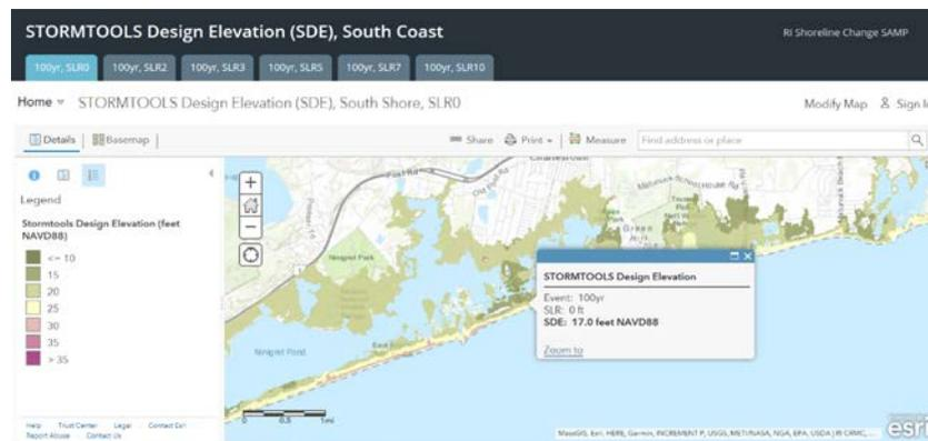
**Figure 8.** Flooding in Charlestown, RI, (see green oval in Figure 2) in the vicinity of Ninigret and Green Hill Ponds for 100-yr, no-SLR case. The insert shows the ability of the point interrogation tool to determine the BFE at the user location selected.
