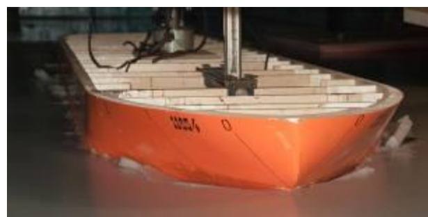
Figure 7. Model test of ahead running.
