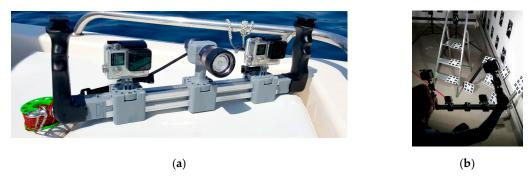
**Figure 16.** Example of the stereo camera rig mounting two GoPro Hero4 Black Edition in their pressure housings (a) and during a pre calibration in the laboratory in the same setup used for Grotta Giusti (underwater lights on the two handles) (b).
