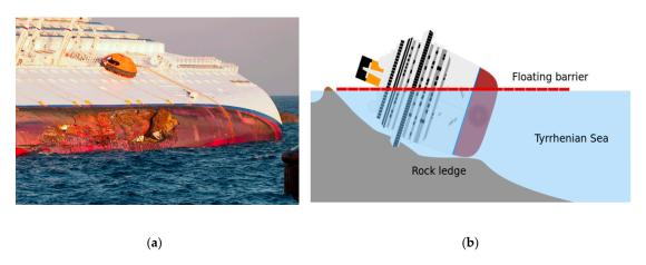
**Figure 5.** The Costa Concordia run aground close to the Giglio Porto, Italy after the collision with a reef on 12th of January 2012 (a) [18]. The shipwreck leaning with the starboard side against the seafloor with a final inclination of about 70 degrees (b) [19].
