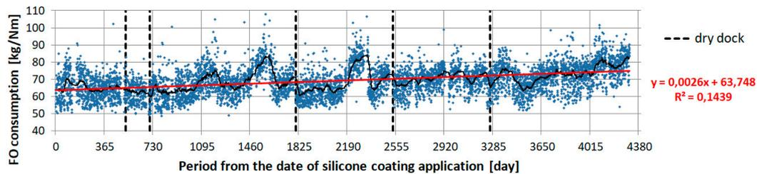
Figure 4. Main engine average fuel consumption for the whole period of study on the route Świnoujście/Trelleborg—both directions.
