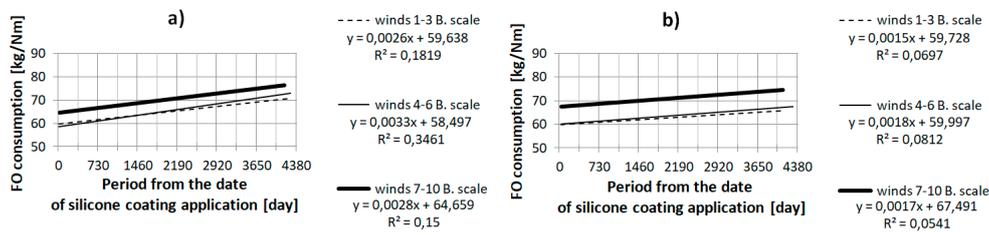
Figure 8. Average fuel consumption—sailing with the wind and wave. Ferry bound for Świnoujście, winds NW/NNW/N (a) and for Trelleborg, winds SE/SSE/S (b).
