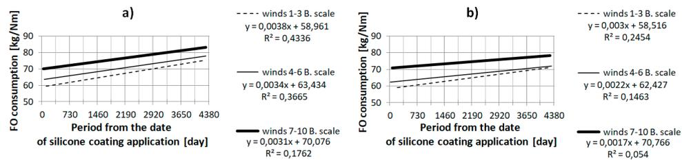
Figure 10. Average fuel consumption—sailing crosswind and large waves from the side. Ferry bound for Świnoujście, winds NE/E/NE/E (a) and for Trelleborg, winds NE/E/NE/E (b).
