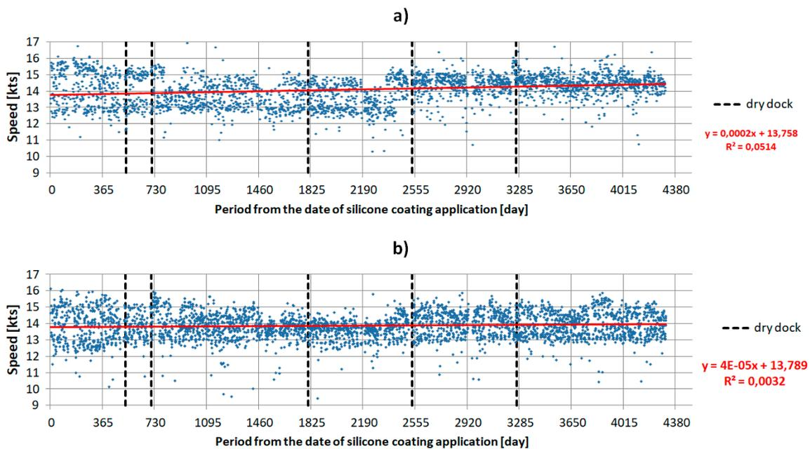
**Figure 6.** Average speed for the entire period of study on the route Świnoujście/Trelleborg—divided into two voyage directions. Ferry bound for Świnoujście (a) and for Trelleborg (b).
