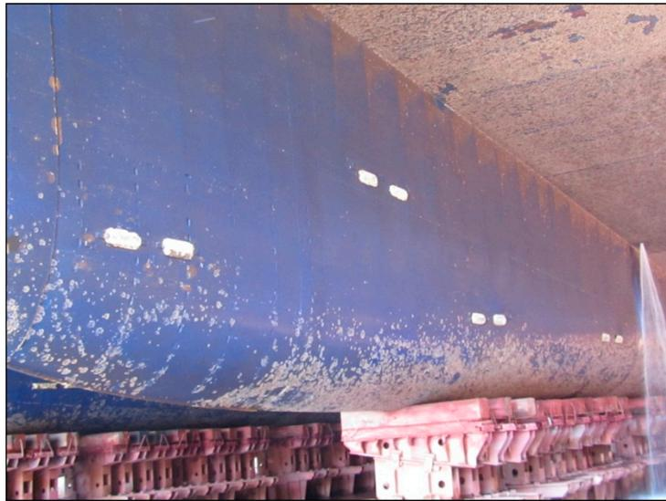
**Figure 1.** View of the silicone coating before high-pressure washing with water at the shipyard in June 2019.
