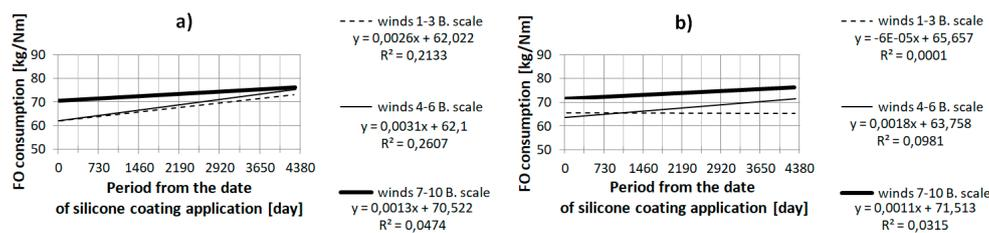
Figure 11. Average fuel consumption—sailing crosswind and small waves from the side. Ferry bound for Świnoujście, winds W/WSW/SW (a) and for Trelleborg, winds W/WSW/SW (b).
