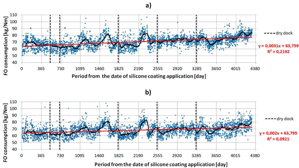
**Figure 7.** Main engine average fuel consumption for the entire period of study on the Świnoujście/Trelleborg route—divided into two voyage directions. Ferry bound for Świnoujście (a) and for Trelleborg (b).
