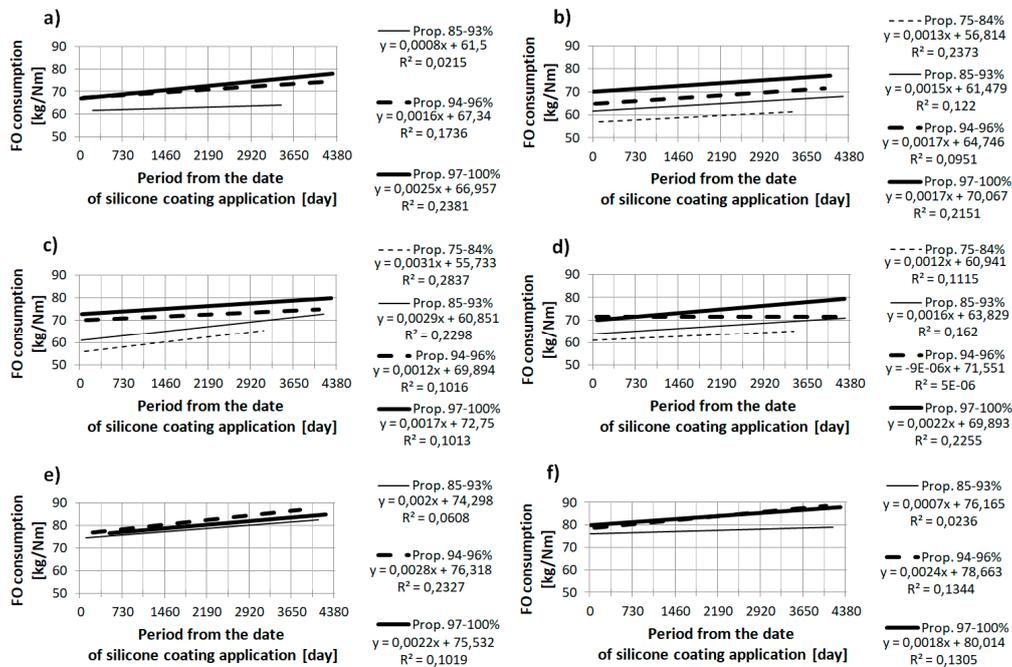
**Figure 13.** Average fuel consumption, sailing against the wind/wave, variable pitch propeller settings. Ferry bound for Świnoujście, winds SE/SSE/S, force: 1–3 B. (a), 4–6 B. (c), 7–10 B. (e) and for Trelleborg, winds NW/NNW/N, force: 1–3 B. (b), 4–6 B. (d), 7–10 B. (f).
