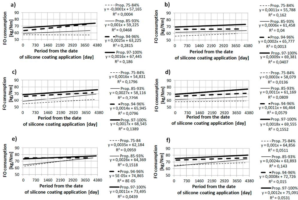
**Figure 12.** Average fuel consumption, sailing crosswind, small waves from the side, variable pitch propeller settings. Ferry bound for Świnoujście, winds W/WSW/SW, force: 1–3 B. (a), 4–6 B. (c), 7–10 B. (e), and for Trelleborg, winds W/WSW/SW, force: 1–3 B. (b), 4–6 B. (d), 7–10 B. (f).
