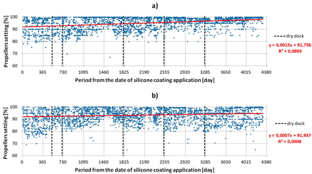
**Figure 5.** Average variable pitch propeller settings for the entire period of study on the Świnoujście/Trelleborg route—divided into two voyage directions. Ferry bound for Świnoujście (a) and for Trelleborg (b).
