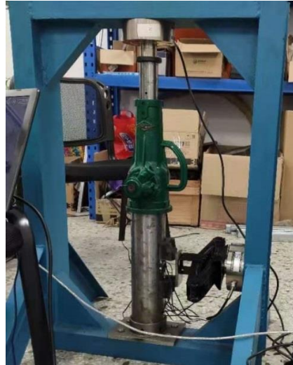
Figure 18. Axial loading of the steel pipe.
