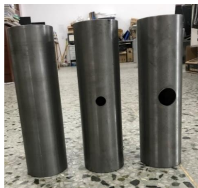
Figure 15. Steel tubes with three different damage holes.
