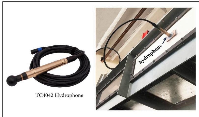
**Figure 5.** Test set-up in the cavitation tunnel at Sharif University of Technology.
