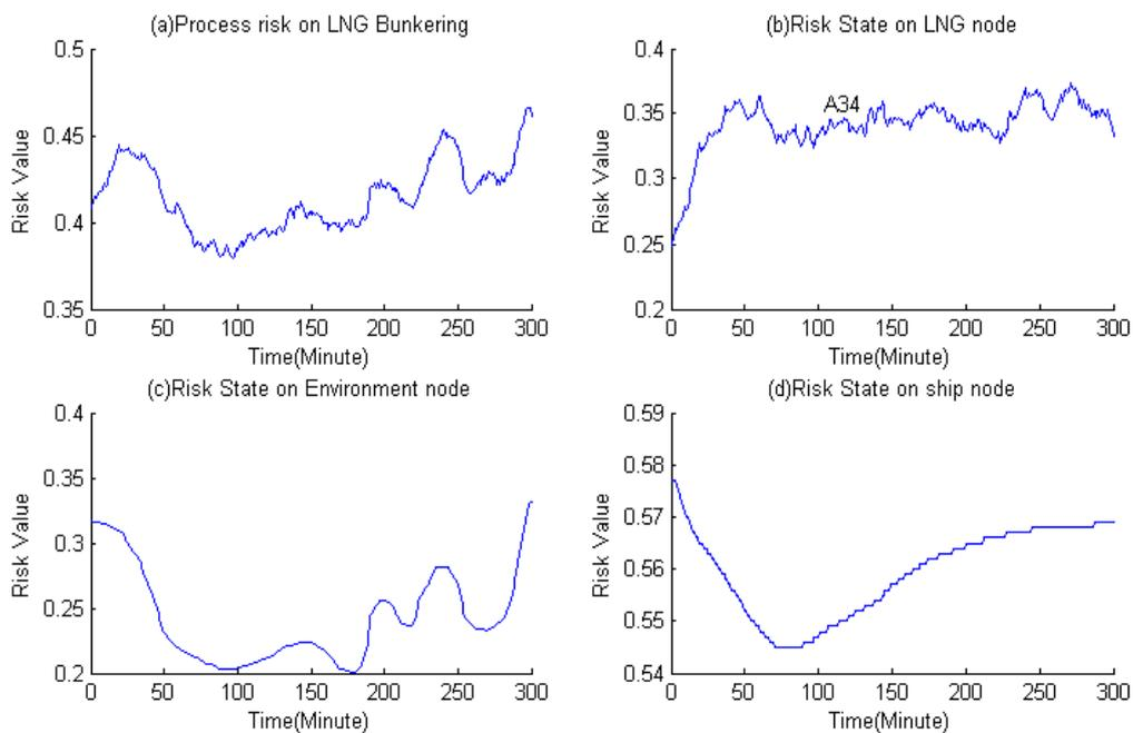
**Figure 7.** Safety level graph on the flange of the connecting pipeline was damaged during the fueling. (a) Process risk on LNG Bunkering. (b) Risk State on LNG node. (c) Risk State on Environment node. (d) Risk State on ship node.
