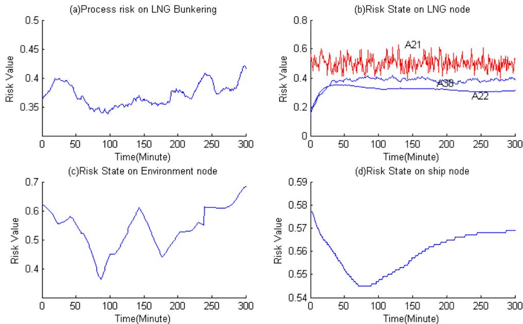
**Figure 5.** Fueling process risk, human-ship-environment sub-system risk. (a) Process risk on LNG Bunkering. (b) Risk State on LNG node. (c) Risk State on Environment node. (d) Risk State on ship node.
