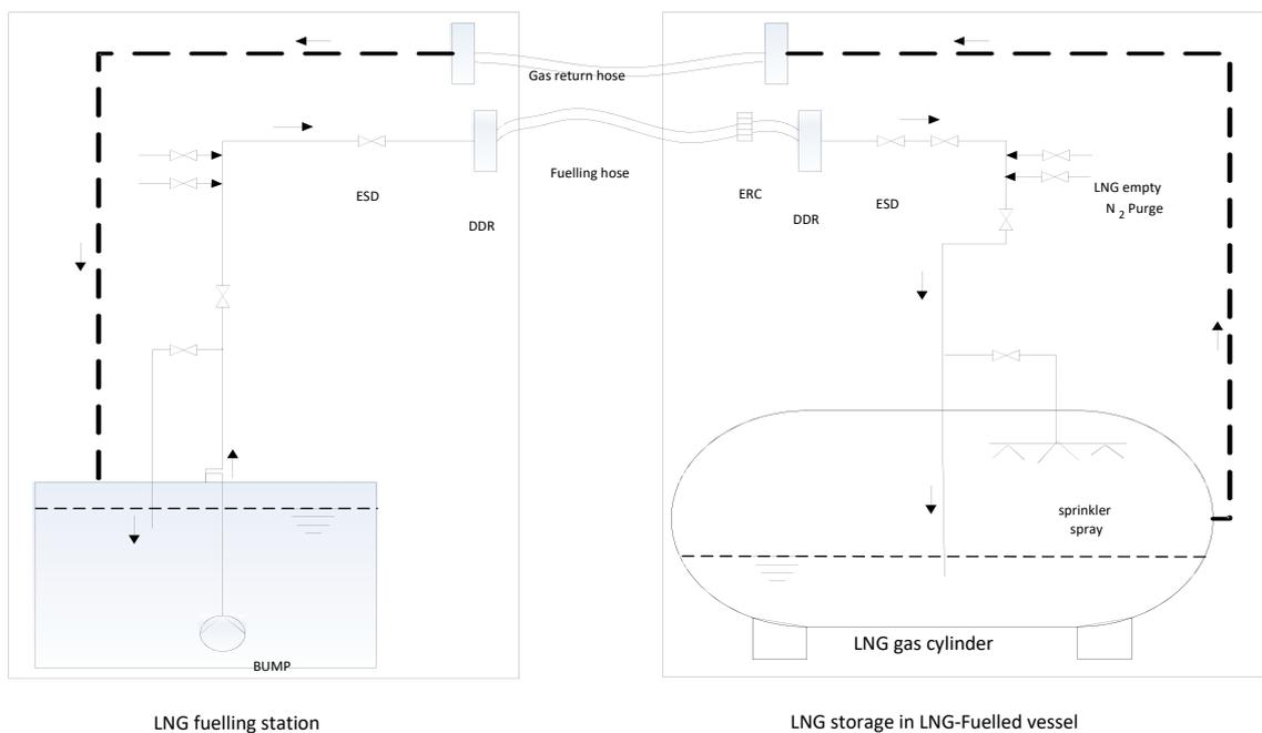
Figure 1. Liquefied nature gas (LNG) intermediary terminal-ship via pipeline (TPS) method.
