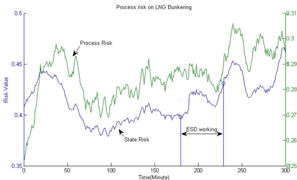
**Figure 8.** Risk evolution on the bunker operation of the LNG-fueled vessel.
