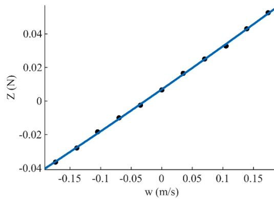
Figure 7. Fitted curve of lateral force Z and linear velocity w.
