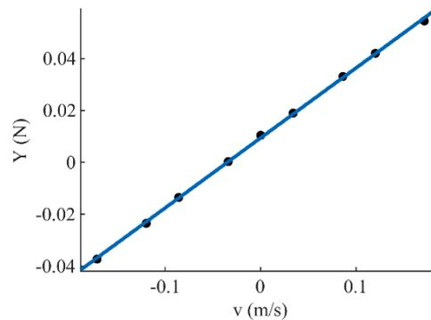
Figure 5. Fitted curve of vertical force  $Y$  and line velocity  $v$ .
