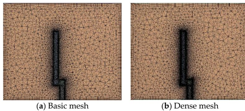
Figure 4. Meshing of manipulator section.
