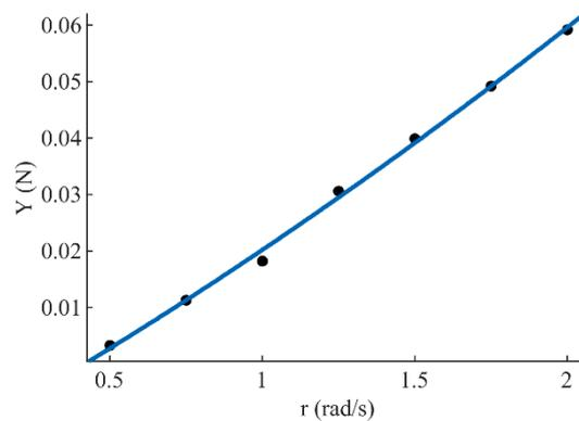
**Figure 9.** Fitted curve of vertical force Y and angular velocity r.
