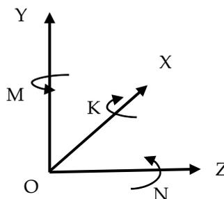
Figure 2. Six-dimensional component of viscous hydrodynamic F.
