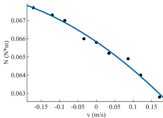
Figure 6. Fitted curve of pitching moment  $N$  and linear velocity  $v$ .
