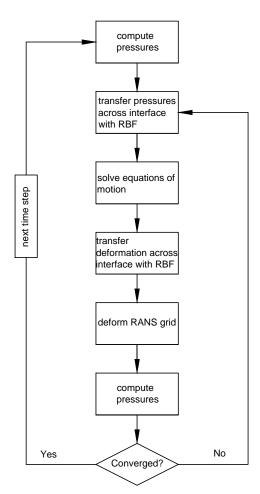
Figure 4. Flow chart of one time step with RANS-FEM coupling.
