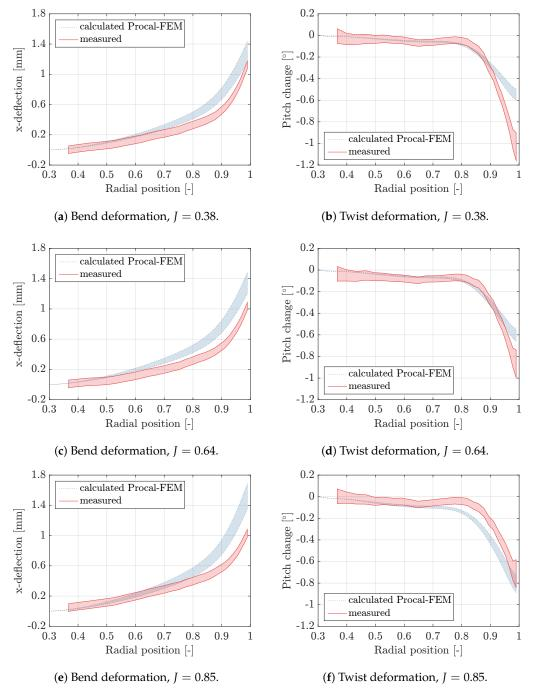
**Figure 17.** Uncertainty intervals for bend (**left**) and twist (**right**) deformations of mid-chord points of propeller 45 blade 1 against the radial position on the blade, for the measured and calculated responses.
