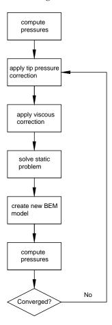
Figure 3. Flow chart of BEM-FEM coupling.
