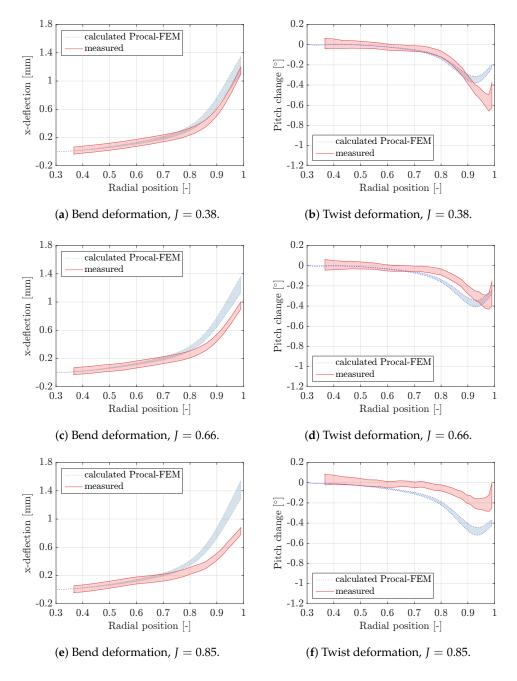
**Figure 18.** Uncertainty intervals for bend (**left**) and twist (**right**) deformations of mid-chord points of propeller 90 blade 2 against the radial position on the blade, for the measured and calculated responses.
