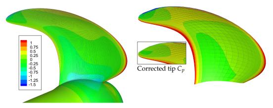
**Figure 12.** Pressure coefficient,  $C_p$ , on the pressure side for J = 0.85, RANS (**left**) BEM (**right**). The insert figure shows the BEM pressure distribution after the tip pressure correction.
