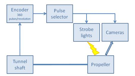
**Figure 13.** Cavitation tunnel set-up diagram.
