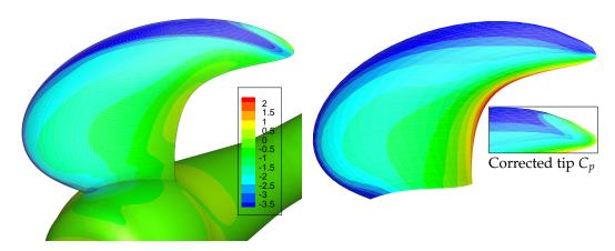
**Figure 7.** Pressure coefficient,  $C_p$ , on the suction side for J = 0.37, RANS (**left**) BEM (**right**). The insert figure shows the BEM pressure distribution after the tip pressure correction.
