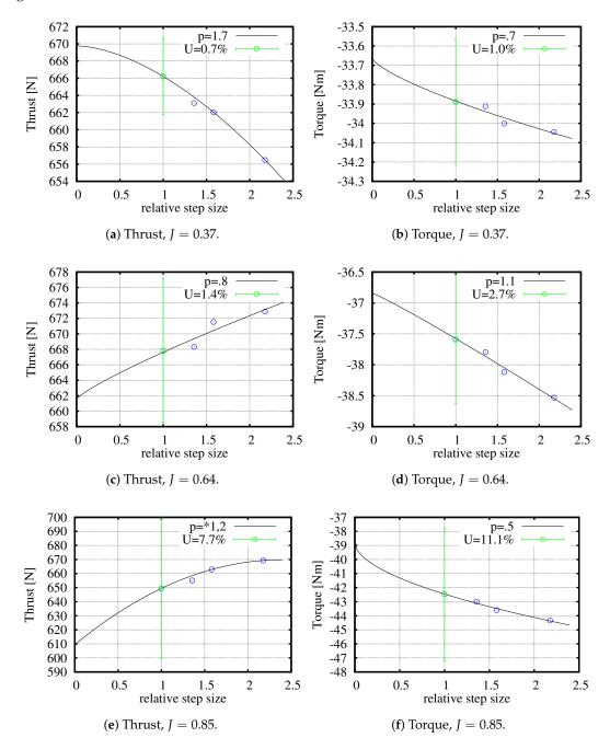
**Figure 2.** Numerical uncertainty of thrust and torque, U and order of accuracy p for various advance ratios.
