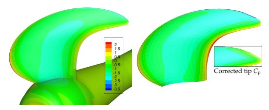
**Figure 11.** Pressure coefficient,  $C_p$ , on the suction side for J = 0.85, RANS (**left**) BEM (**right**). The insert figure shows the BEM pressure distribution after the tip pressure correction.
