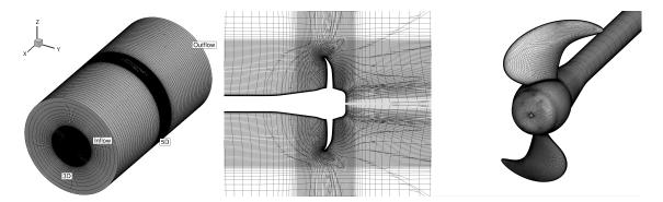
Figure 1. Domain and grid for Reynolds-averaged-Navier-Stokes computations.
