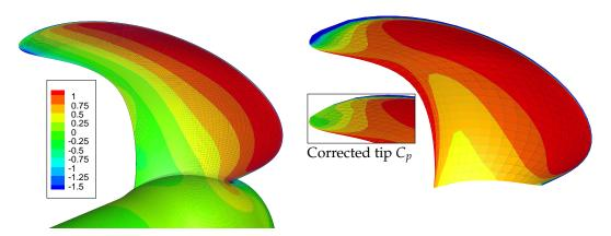
**Figure 8.** Pressure coefficient,  $C_p$ , on the pressure side for J = 0.37, RANS (**left**) BEM (**right**). The insert figure shows the BEM pressure distribution after the tip pressure correction.
