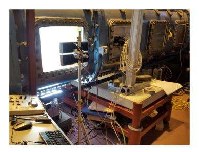
Figure 15. Picture of the cavitation tunnel test set-up.
