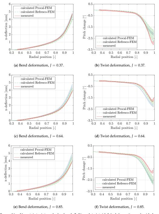
**Figure 16.** Uncertainty intervals for bend (**left**) and twist (**right**) deformations of mid-chord points of epoxy propeller blade 1 against the radial position on the blade, for the measured and calculated responses.
