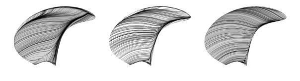
**Figure 6.** Limiting streamlines on propeller suction side for J = 0.37, J = 0.64 and J = 0.85.
