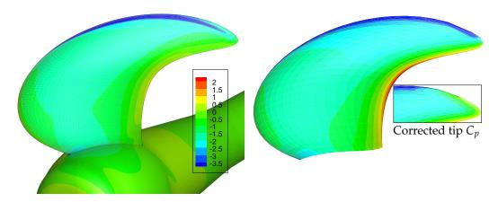
**Figure 9.** Pressure coefficient,  $C_p$ , on the suction side for J = 0.64, RANS (**left**) BEM (**right**). The insert figure shows the BEM pressure distribution after the tip pressure correction.
