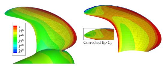
**Figure 10.** Pressure coefficient,  $C_p$ , on the pressure side for J = 0.64, RANS (**left**) BEM (**right**). The insert figure shows the BEM pressure distribution after the tip pressure correction.
