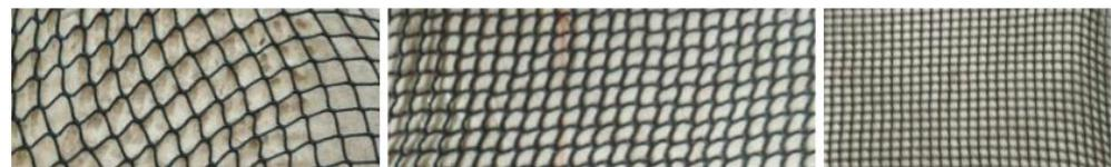
**Figure 7.** Different types of nets; knot distances of 30 mm (left), 20 mm (center), and 10 mm (right).
