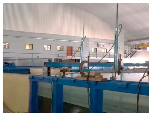
**Figure 2.** Resistive-type sensors used to measure incident and reflected wave heights.
