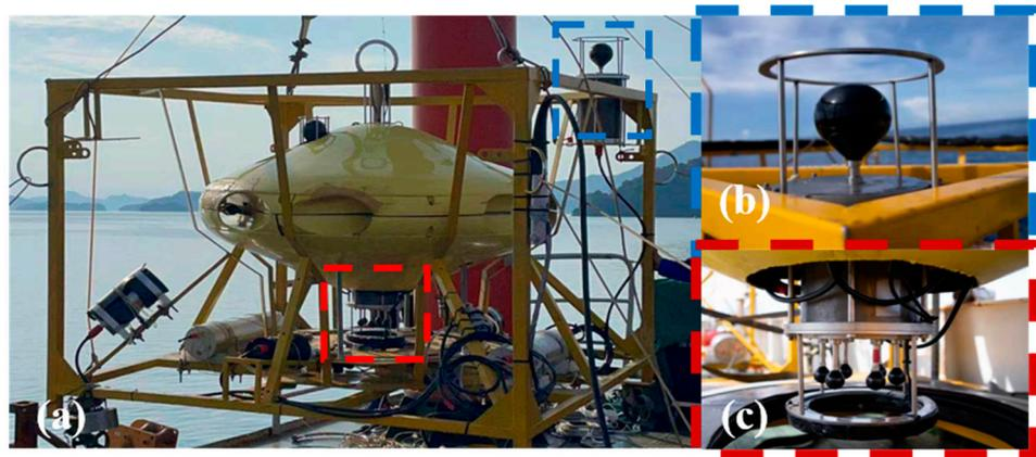
**Figure 2.** Pictures of the AUV and the iUSBL system. (a) Disc-shaped AUV deployed with base station; (b) acoustic beacon is mounted on the base station and broadcasts positioning signals; (c) the iUSBL receiving array mounted on the bottom of the AUV.
