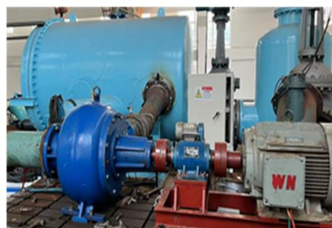
(a) Test bench of model pump
