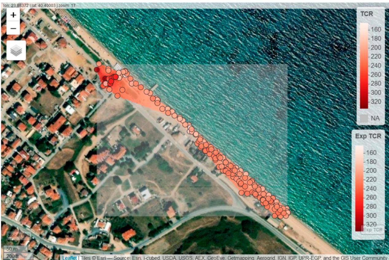
Figure 4. The radioactivity distribution of the total counting rate using interpolation methods (for the Ierissos area). The experimental data derived TCR are depicted with circles.
