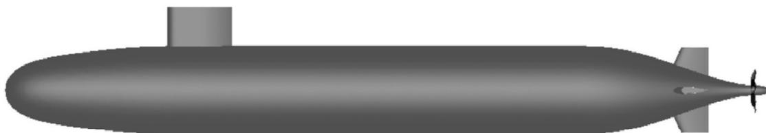
**Figure 2.** DARPA SuboffAFF8 model with propeller.
