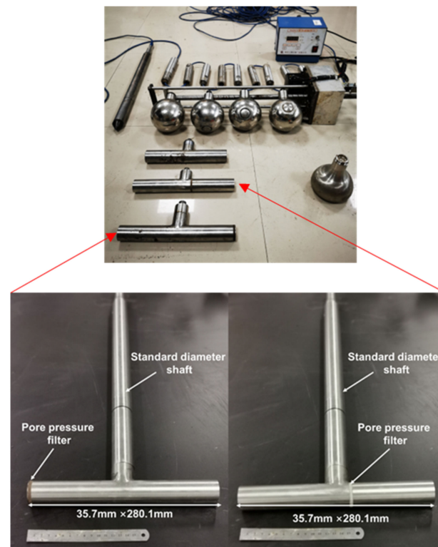
Figure 29. Piezo full-flow penetrometers (in this paper).
