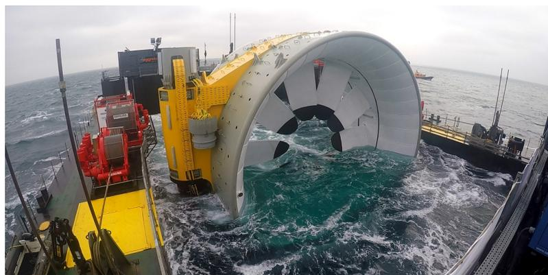
(b) OpenHydro tidal stream turbine (direct-drive turbine).
