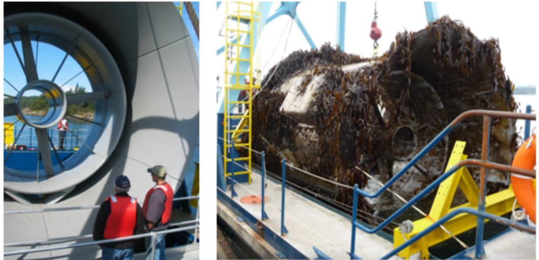
**Figure 4.** The Clear Current Company tidal stream turbine: Immersed in September 2006 and retrieved in October 2011 due to loss of performance. Reproduced from [20].
