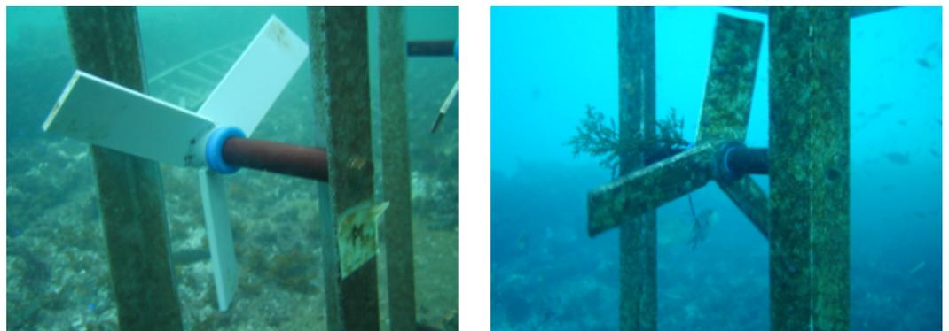
**Figure 5.** Illustration of the corrosion acceleration due to biofouling. Courtesy of Prof. Yusaku Kozuka [27].
