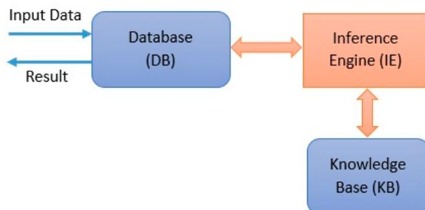
Figure 1. Basic expert system architecture.
