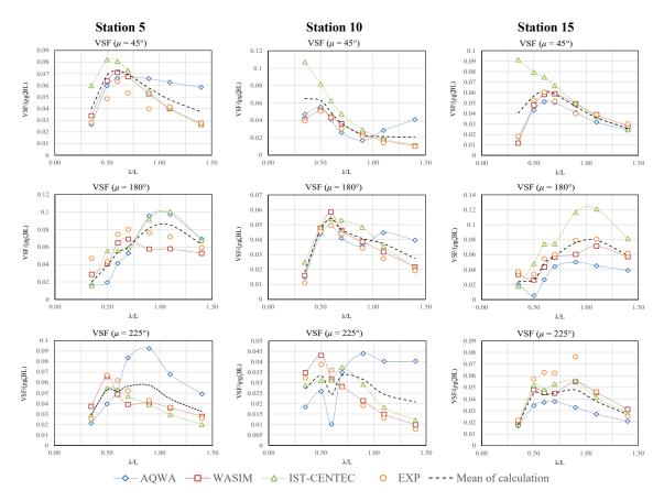
**Figure 6.** Calculated and measured nondimensional vertical shear forces (VSF) on the Flokstra container ship at Fr = 0.245.
