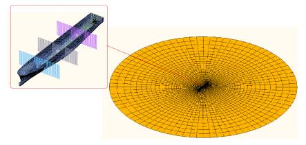
Figure 4. Applied meshes in WASIM numerical simulation.
