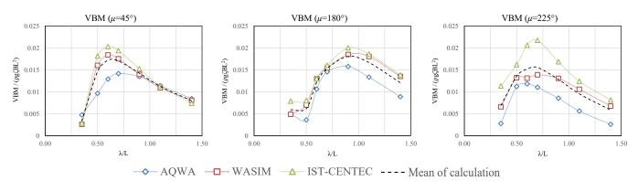
**Figure 12.** Calculated nondimensional vertical bending moment (VBM) at station 10 in the Flokstra ship at Fr = 0.1.
