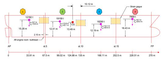
Figure 2. Mass distribution of the Flokstra ship as reconstructed from data in reference [88].
