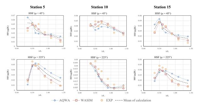
**Figure 7.** Calculated and measured nondimensional horizontal shear forces (HSF) on the Flokstra ship at Fr = 0.245.
