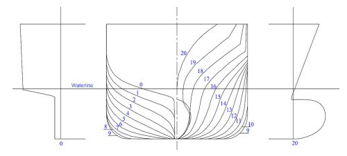
Figure 1. The body plan of the container ship Flokstra as reconstructed from data in reference [88].
