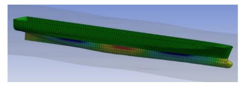
Figure 3. Discretized mesh in AQWA numerical simulation.
