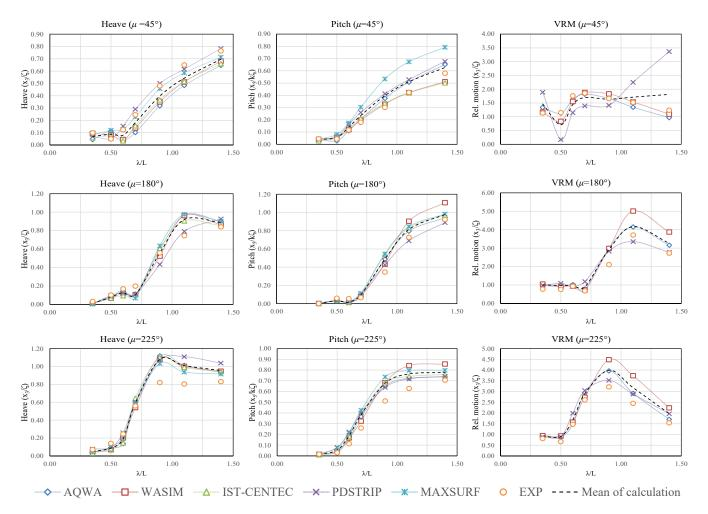
**Figure 5.** Calculated and measured nondimensional motions (Heave, Pitch, and VRM) of the Flokstra ship at Fr = 0.245.
