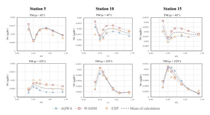
**Figure 10.** Calculated and measured nondimensional torsional moments (TM) of the Flokstra container ship at Fr = 0.245.
