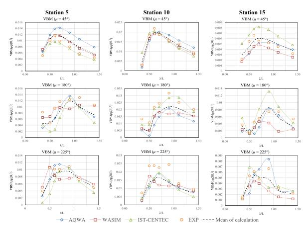
**Figure 8.** Calculated and measured nondimensional vertical bending moments (VBM) of the Flokstra ship at Fr = 0.245.
