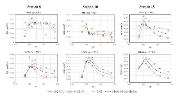
**Figure 9.** Calculated and measured nondimensional horizontal bending moments (HBM) of the Flokstra ship at Fr = 0.245.
