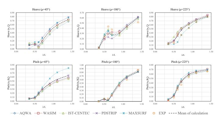
**Figure 11.** Calculated and measured nondimensional motions (Heave and Pitch) of the Flokstra ship at Fr = 0.1.
