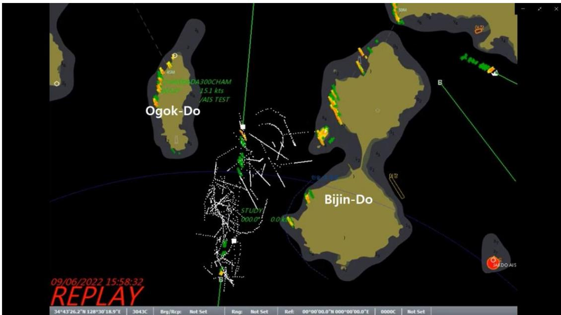
Figure 9. Screen-grab of the Tongyong coastal Vessel Traffic Service (VTS) radar screen showing the experimental track.
