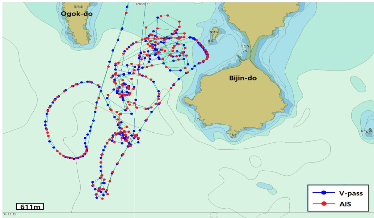
Figure 3. Comparison of the AIS and V-pass data.
