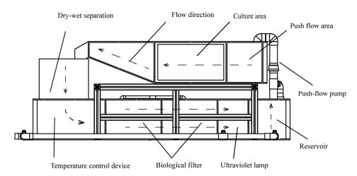
Figure 1. Circulating water culture tank.
