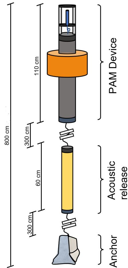
**Figure 2.** Details of the mooring line experimental setup. It consists of an anchor, an acoustic release, and the passive acoustic recorder integrated into a ringed buoy.
