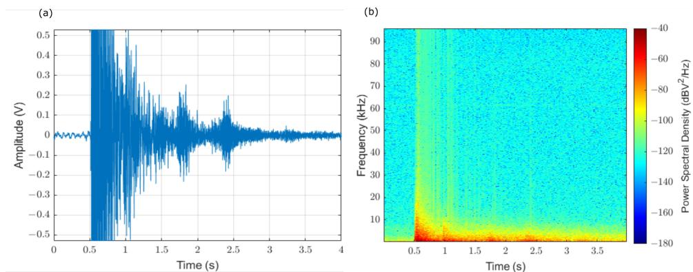
**Figure 3.** Details of an underwater explosion event recorded (a) in the temporary domain, with the Y-axis representing the output voltage of the electroacoustic chain and (b) in the time–frequency domain (obtained in dBV<sup>2</sup>/Hz). It is possible to observe how the acoustical signal exceeded the allowable full-scale input ( $\pm\sqrt{2} * 0.375$  V) of the SAMARUC analog-to-digital converter.
