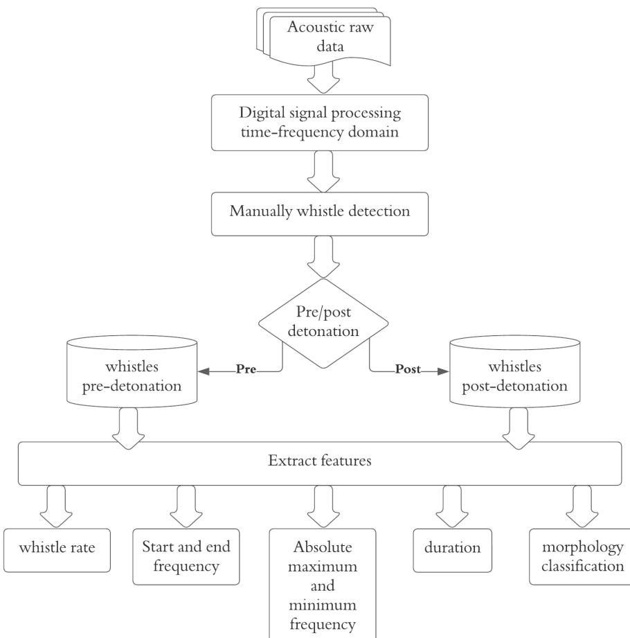
**Figure 5.** Analysis workflow diagram.
