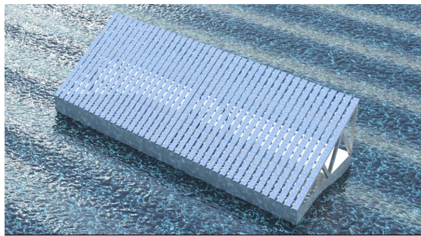
Figure 1. Pontoon-type floating structure supporting arrays of photovoltaic panels.
