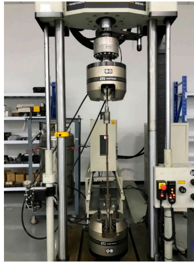
Figure 6. Fatigue test equipment for rusted steel strand.
