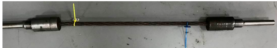
Figure 7. Assembly diagram of steel strand and clamp for fatigue test.
