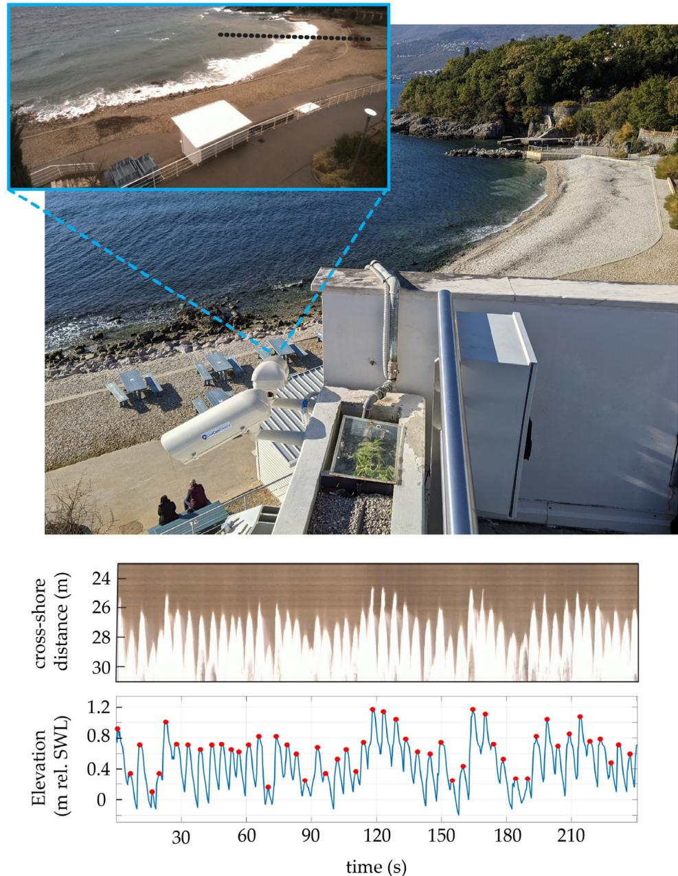
**Figure 3.** Position of the video monitoring system at the edge of the swimming pool complex at the beach site, one camera per beach cell; observed pixel cross-section of the acquired video gives the cross-shore distance time series of wave uprush, which ultimately results in the water elevation time series on the shoreline.
