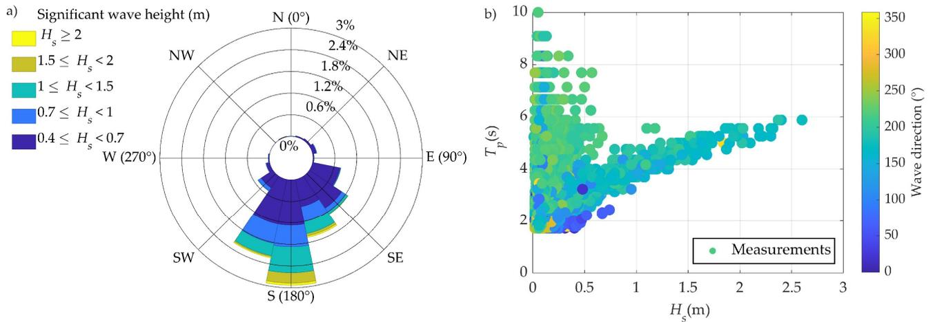
**Figure 5.** (a) The wave rose for the wave buoy during the measuring period (December 2019 to April 2021) in front of the Ploče beach; (b) scatter plot of significant wave heights against peak wave periods during the measuring period with wave direction as coloring.
