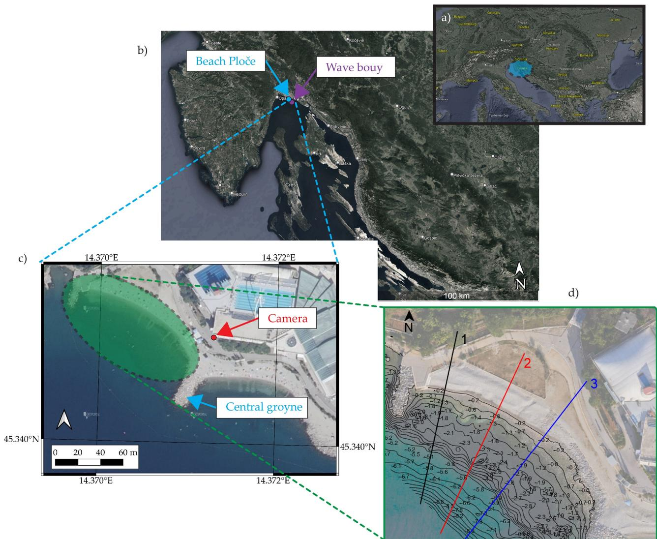
**Figure 1.** (a) Map of Europe; (b) map of the northern Adriatic Sea indicating the study site and wave bouy; (c) beach Ploče with the indicated camera and central groyne position; (d) Positions of cross shore profiles (1, 2, and 3) selected for the runup analysis.
