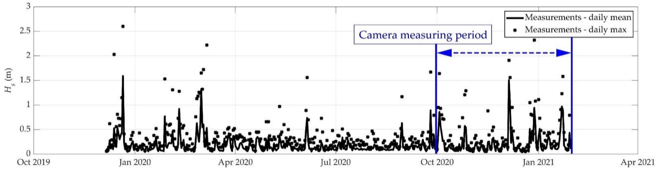
**Figure 4.** The daily averaged and daily maximum significant wave height values observed in front of the Ploče beach during the measuring period of December 2019 to April 2021; the camera observation period (wave runup measurements) is indicated with blue vertical lines.
