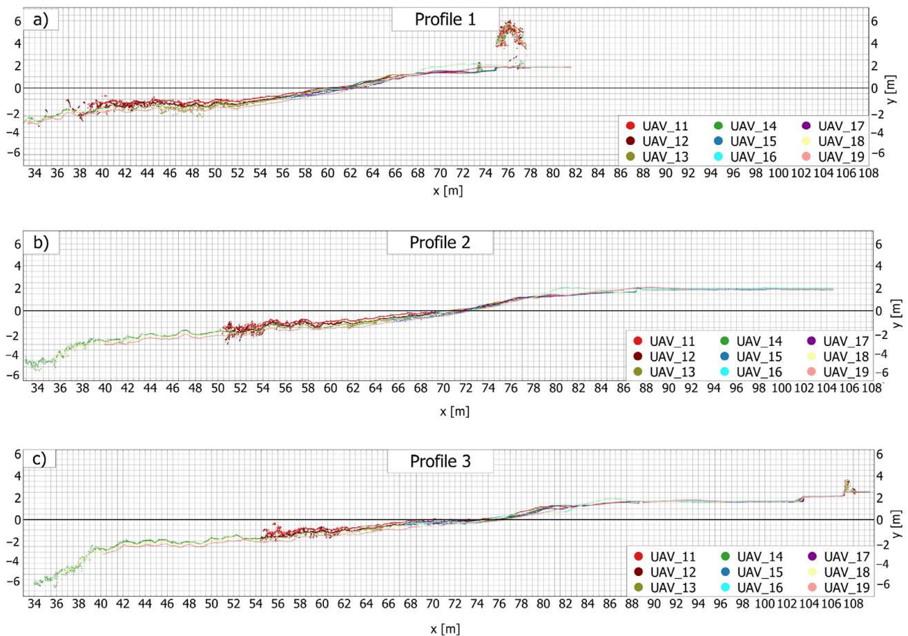
**Figure 2.** Cross shore profiles selected for the runup analysis; (a) the western profile position, which is shown on Figure 1d as profile 1; (b) the centerline profile position, which is shown on Figure 1d as profile 2; (c) the eastern profile position, which is shown on Figure 1d as profile 3; table showing the nine associated UAV surveys between 1 October 2020 and 26 February 2021 is in Appendix A.
