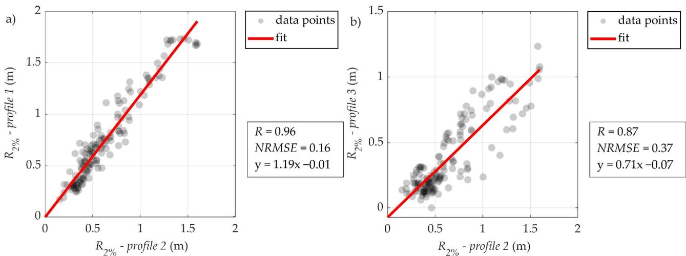
**Figure 11.** (a) Relationship between the wave runup,  $R_{2\%}$ , measured on the centerline profile (profile 2 in Figure 1d) and westward profile (profile 1 in Figure 1d); (b) Relationship between the wave runup,  $R_{2\%}$ , measured on the centerline profile (profile 2 in Figure 1d) and eastward profile (profile 3 in Figure 1d).
