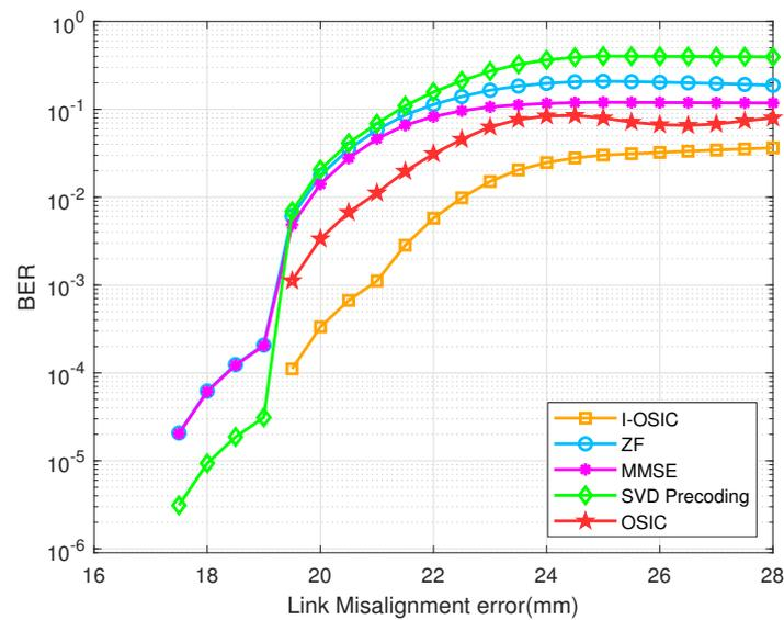
**Figure 13.** The system BER versus the link misalignment error when SNR is 30 dB.
