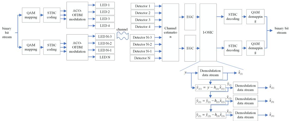
Figure 2. MIMO ACO-OFDM STBC system block diagram.
