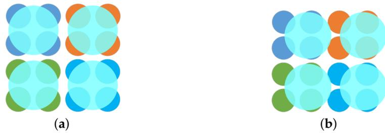
**Figure 8.** Schematic diagram of imaging spot distribution under different link misalignments. (a) The degree of link misalignment is small. (b) The degree of link misalignment is large.
