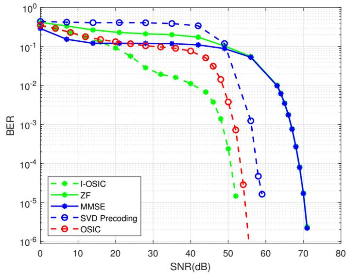
Figure 12. System BER performance when the link misalignment error is 18 mm.
