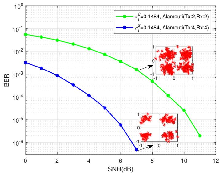
**Figure 9.** BER curves of systems with different diversity orders under weak turbulence conditions.
