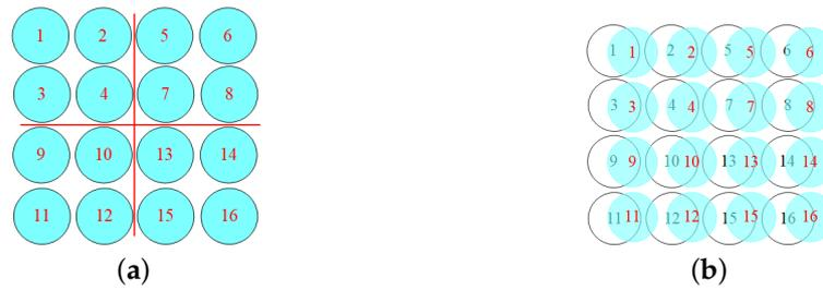
**Figure 3.** Image spot distribution diagram at the receiver. (a) Transceiver alignment. (b) The transceiver link misalignment.
