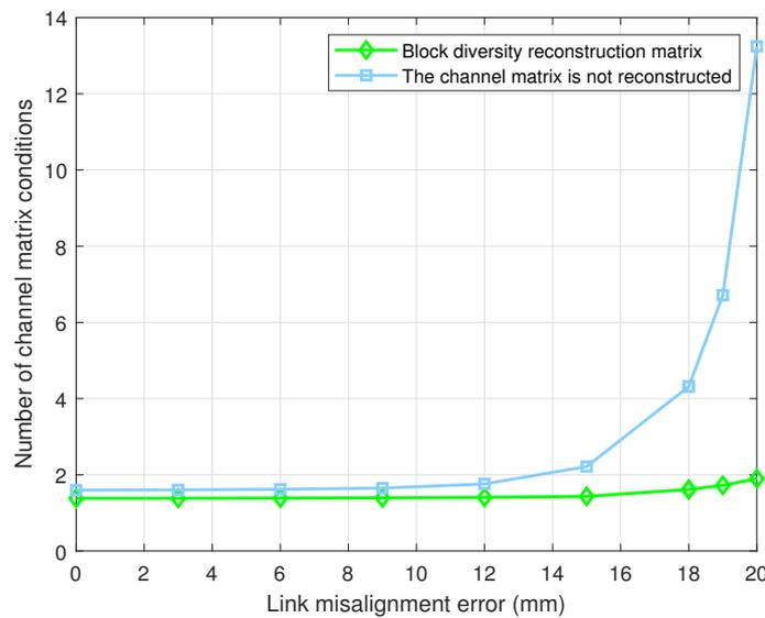
Figure 7. The conditions number of  $\mathbf{H}$  versus the link misalignment error  $\Delta x$  in turbulent environment.
