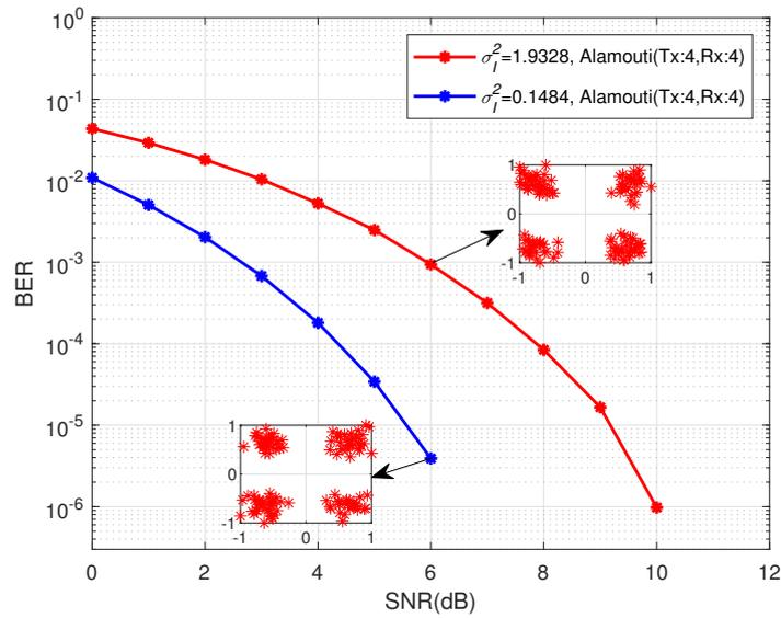
Figure 10. BER curves of 4 × 4 STBC coding system under different turbulent environments.
