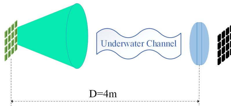
**Figure 1.** Model of underwater imaging optical communication system.
