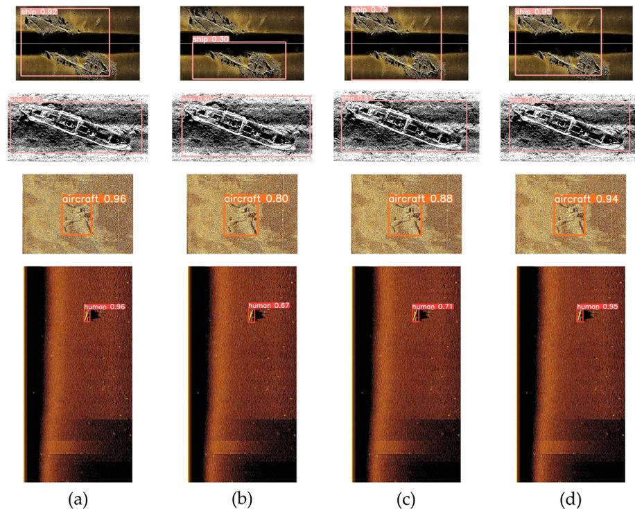
**Figure 14.** Some representative detection results of four models using Jetson Nano. (a) YOLO-slimming; (b) YOLOv5-s; (c) YOLOv6-s; (d) YOLOv7-tiny.
