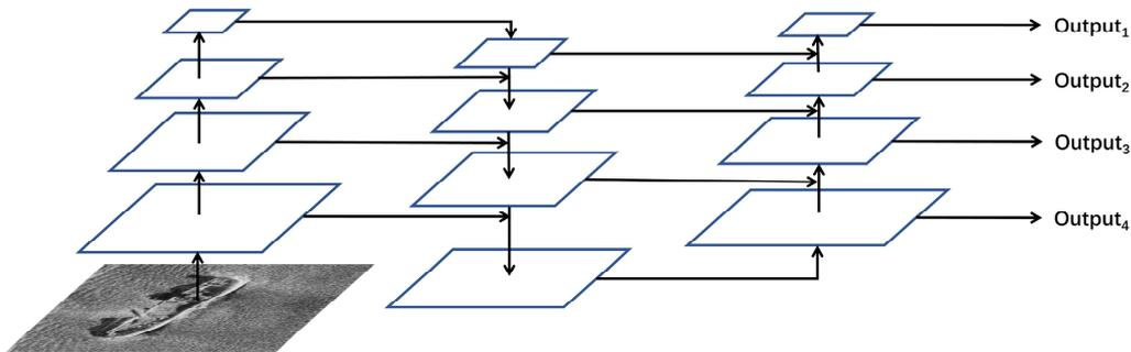
Figure 4. Illustration of a PAN (parallelograms are feature maps).
