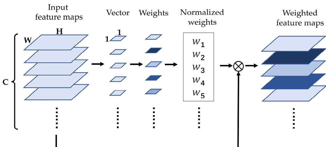
Figure 5. Channel-excitation feature encoder.  $\otimes$  indicates element-wise multiplication.
