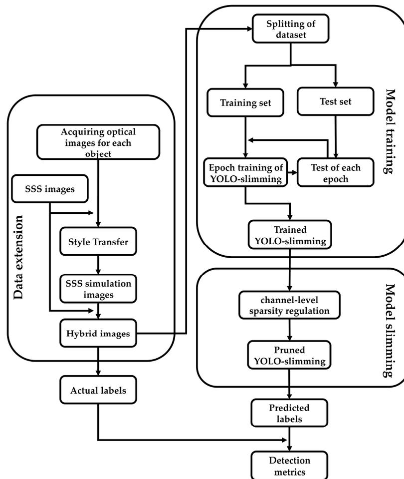
Figure 1. Workflow diagram of YOLO-slimming.
