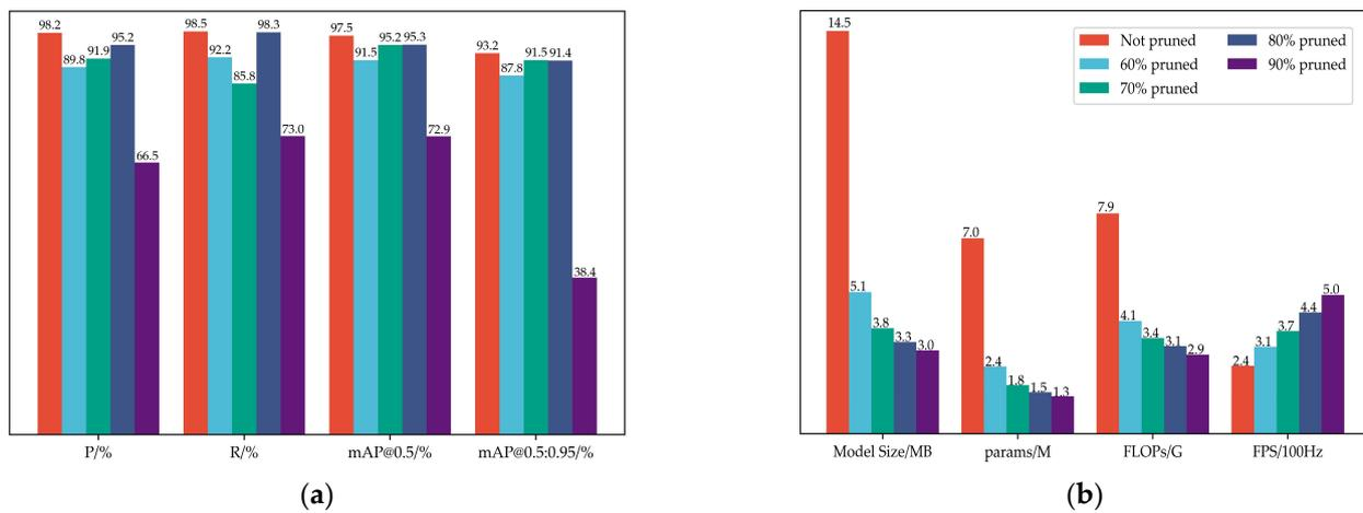
Figure 13. Performance of YOLO-slimming with different pruning ratios. (a) Accuracy; (b) Complexity.
