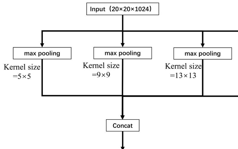
Figure 3. The structure of the SPP.
