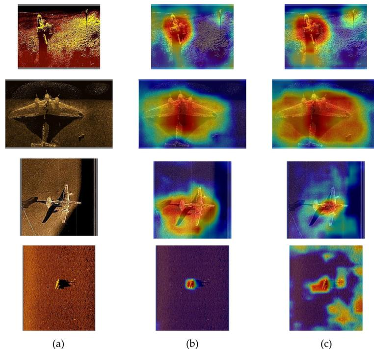
**Figure 12.** Detection results with heatmap. (a) Original images; (b) detection with a CE feature encoder; and (c) detection of the original network.
