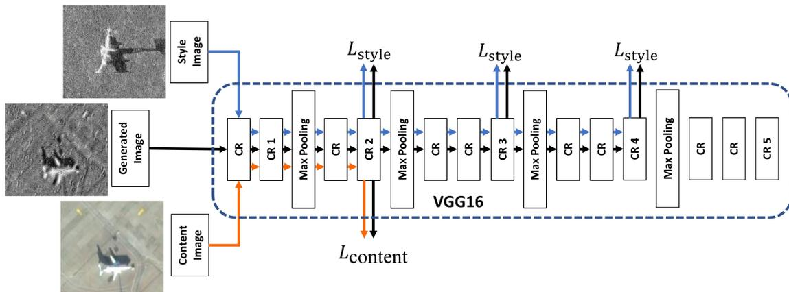
Figure 6. One loop of image ST with VGG16 (generated image is random noise before the first loop).
