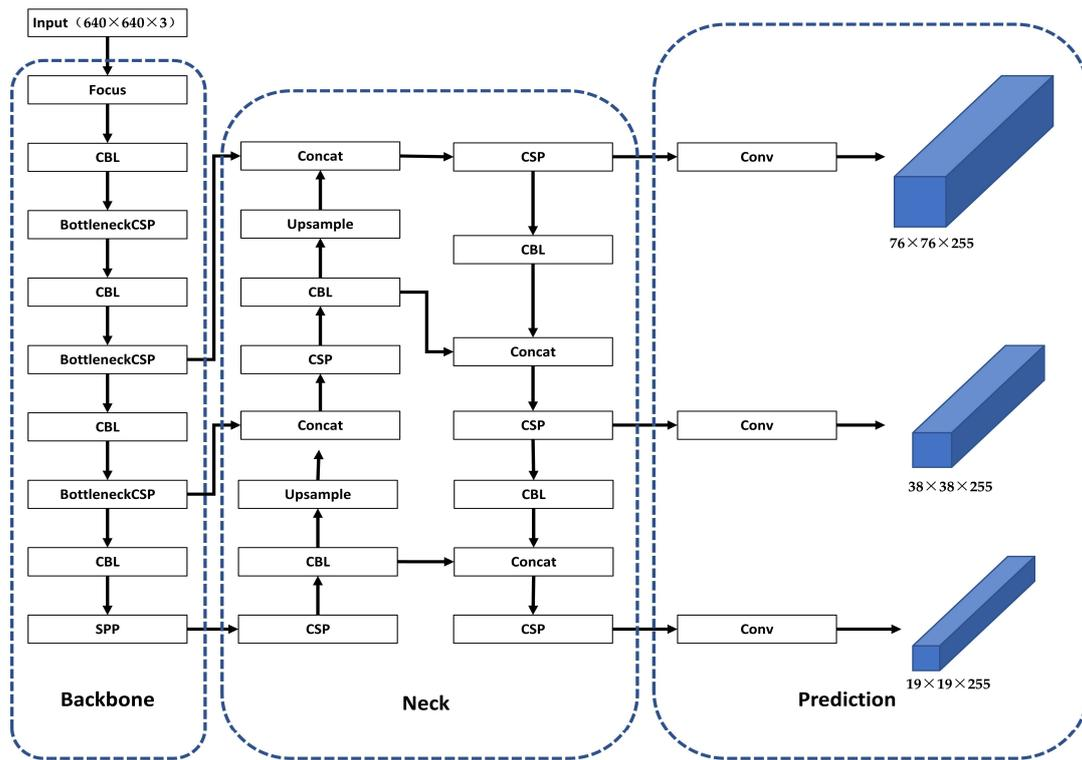
Figure 2. The structure of YOLOv5.
