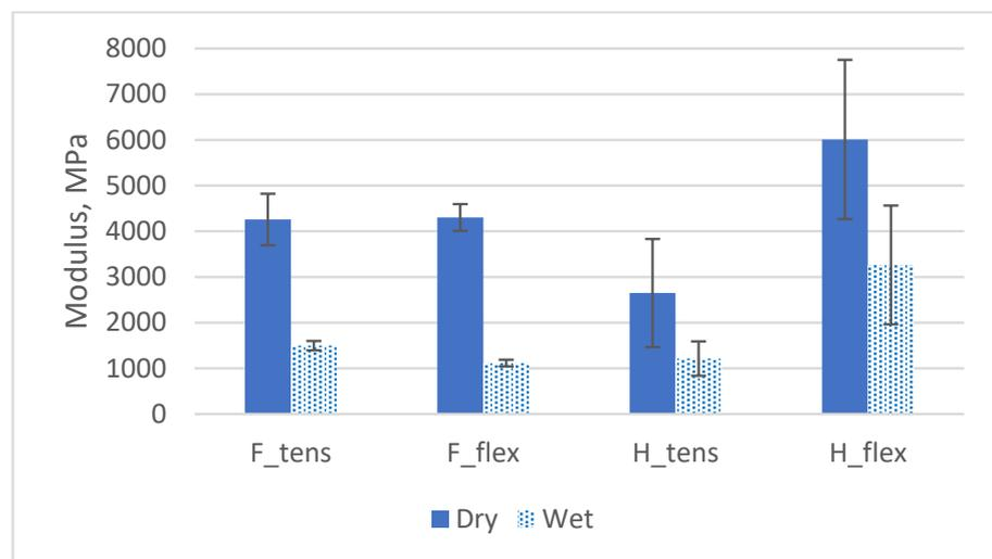
**Figure 5.** Effect of seawater treatment on tensile (tens) and flexural (flex) modulus of flax/epoxy (F) and hemp/epoxy (H).
