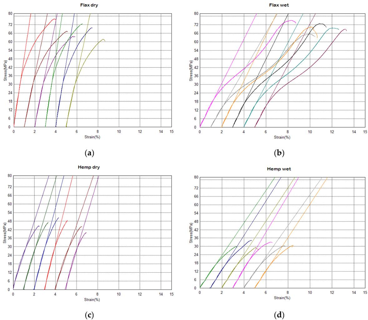
**Figure 2.** Stress–strain test results for 6 samples under tensile load: (a) flax/epoxy dry, (b) flax/epoxy wet, (c) hemp/epoxy dry, and (d) hemp/epoxy wet. (The 1% shift along the x-axis is intentional and allows better clarity of the results. Each sample is presented using different colour).
