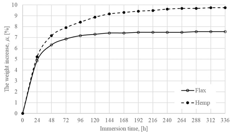
**Figure 1.** The seawater uptake of flax/epoxy and hemp/epoxy.
