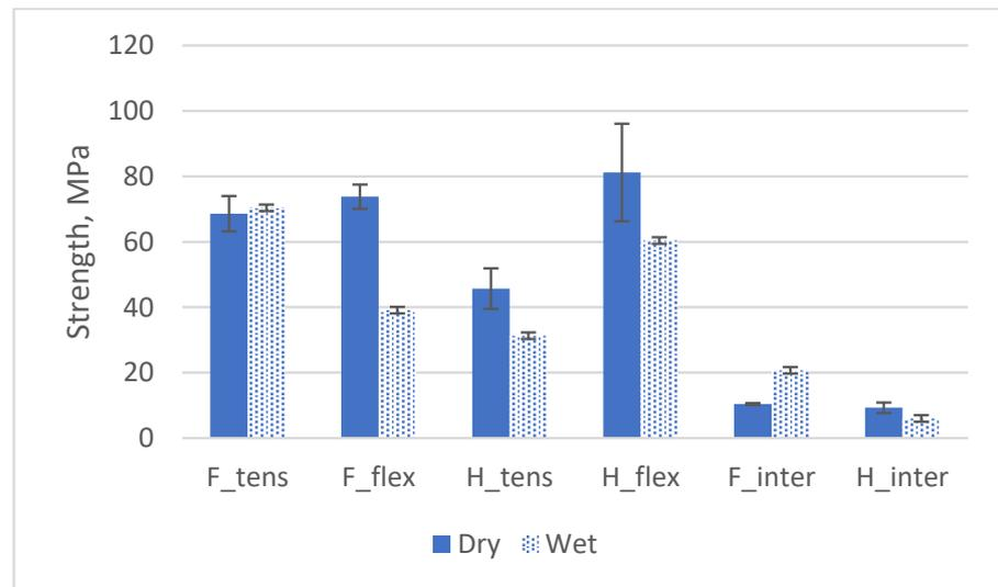
**Figure 4.** Effect of seawater treatment on tensile (tens), flexural (flex), and apparent interlaminar shear strength (inter) of flax/epoxy (F) and hemp/epoxy (H).
