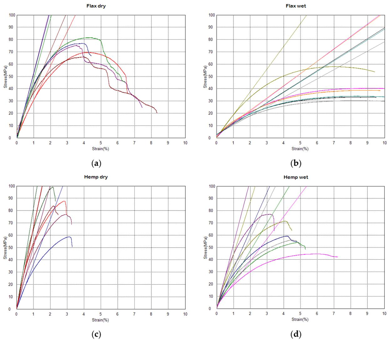
**Figure 3.** Stress–strain test results for 6 samples under flexural load: (a) flax/epoxy dry (b) flax/epoxy wet, (c) hemp/epoxy dry, and (d) hemp/epoxy wet. (Each sample is presented using different colour).
