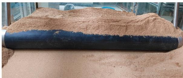
**(a)**  $7D$  position lateral displacement (test)
