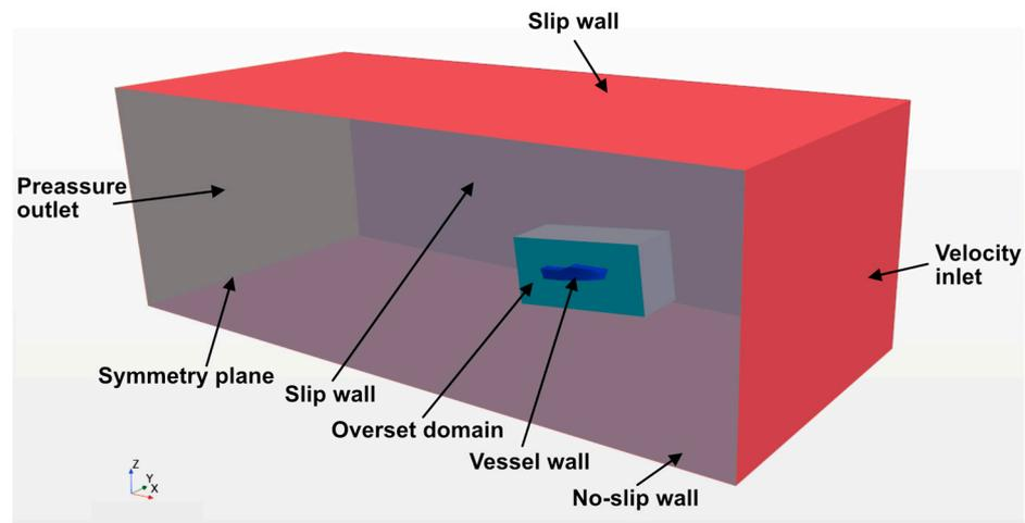
**Figure 6.** Computational domain boundary conditions.
