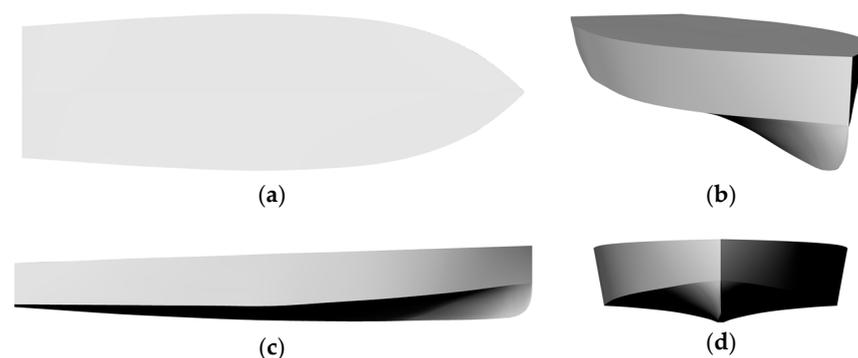
**Figure 1.** CAD model for Hull 2743 from Series 50: (a) top view, (b) isometric view (c) profile view and (d) front view.
