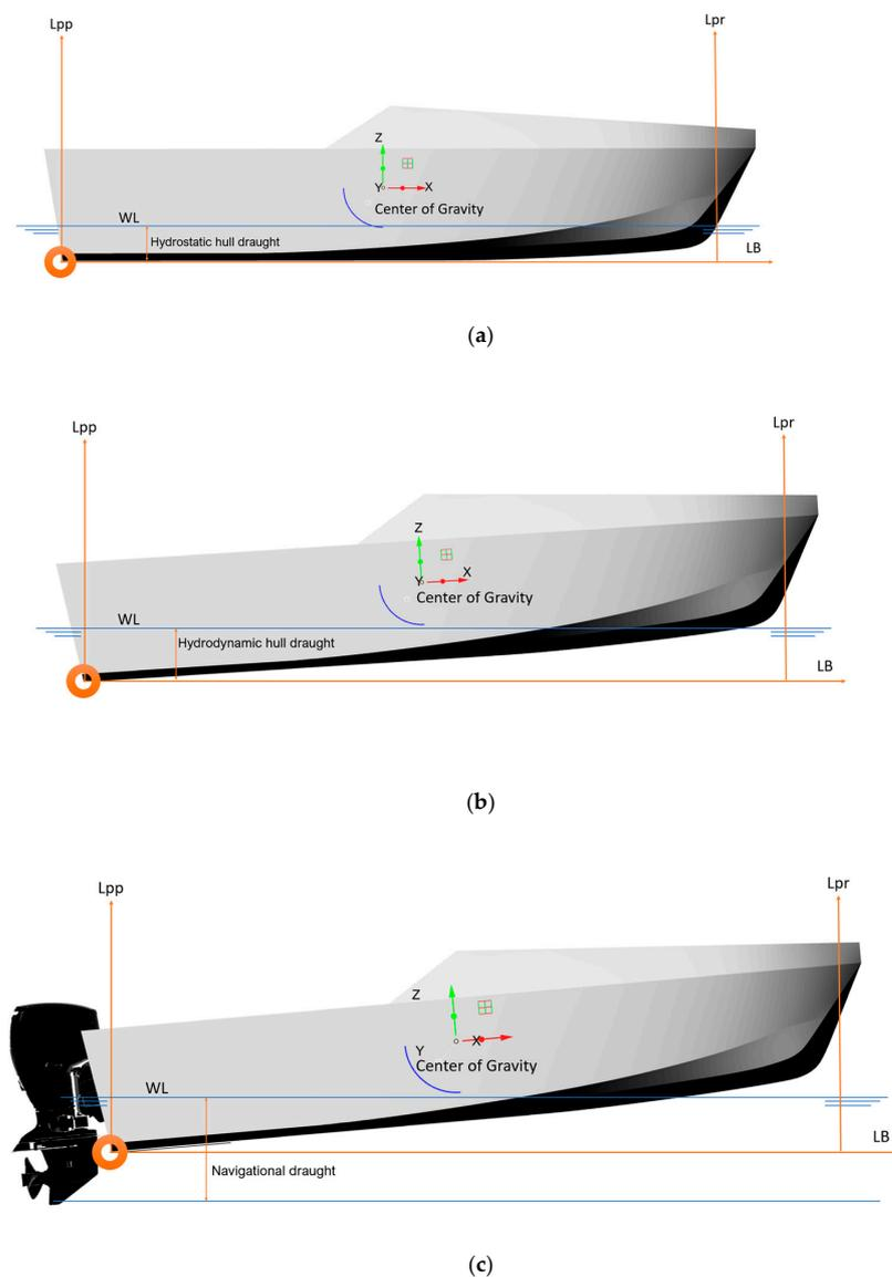
**Figure 2.** Graphical scheme for defining draft/draughts in a craft: (a) hydrostatic hull draught, (b) hydrodynamic hull draught, and (c) navigational draught.
