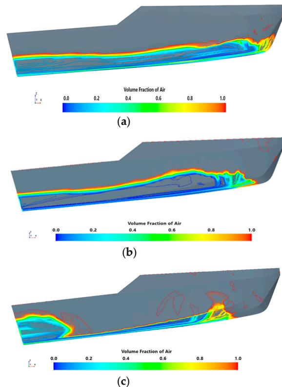
**Figure 8.** Profile view of wetted surface at different hull speeds for RRC: (a) 9 Knots, (b) 12 Knots, and (c) 15 Knots.
