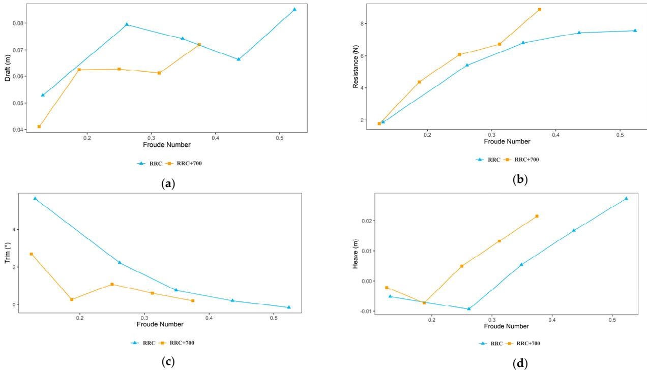
**Figure 10.** Comparison of the RRC and RRC+700 with Froude Numbers (Numerical-CFD Study): (a) draft, (b) resistance, (c) trim, and (d) heave.
