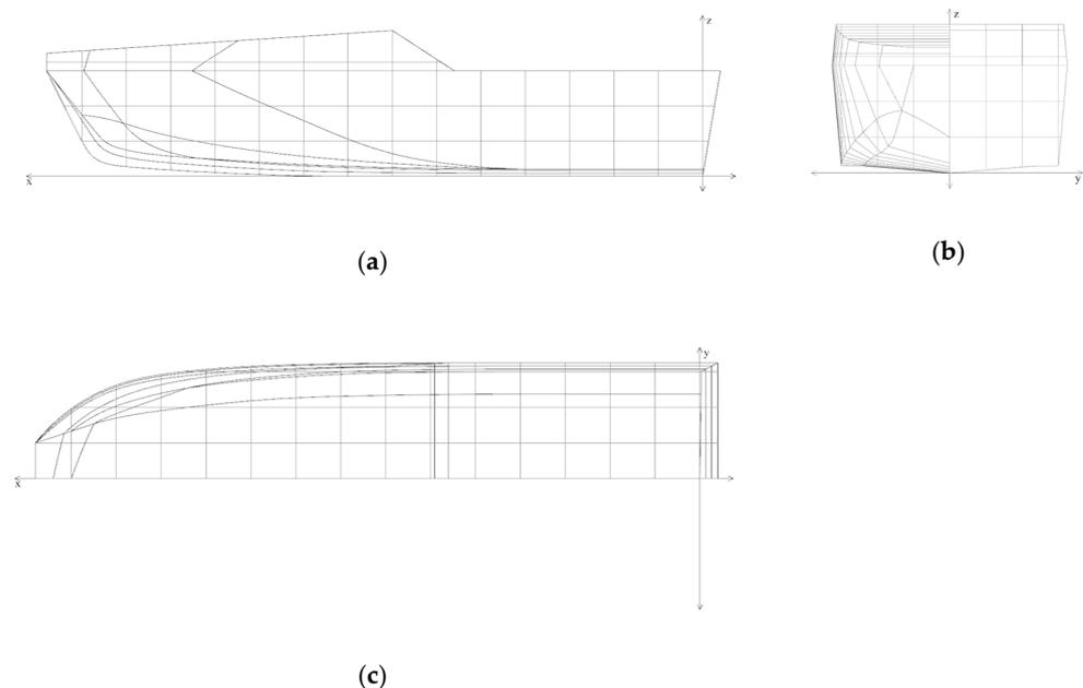
**Figure 3.** Lines and forms of the RRC hull: (a) profile view, (b) buttock line view, and (c) waterplane view.
