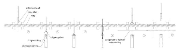
Figure 5. Schematic diagram of kelp seedling clipping.
