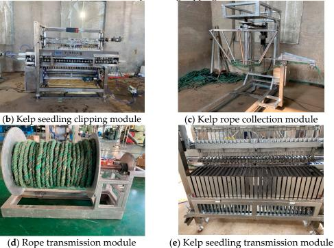
Figure 3. Automatic kelp seedling clipping machine.
