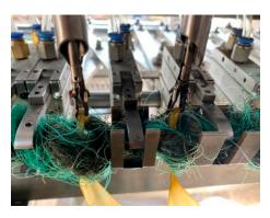
Figure 8. Kelp seedling clipping test.
