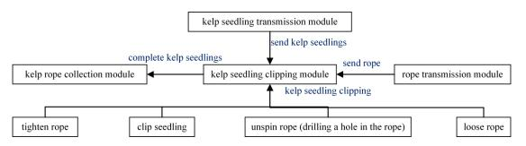
Figure 4. System flow chart for kelp seedling clipping.
