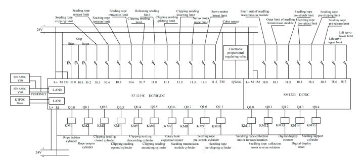
**Figure 6.** Circuit diagram. Note: L+ and M are 24 VDC power inputs, 1 M and 2 M are common terminals, I0.0~I1.5 and I8.0~I8.7 are input button and limit switch, AI0 is analog input, Q0.0~Q1.1 and Q8.0~Q8.4 are control outputs, SIEMENS V90 is a Siemens V90 inverter, KTP700 Basic is a Siemens KTP series touch screen, LAN0 and LAN1 are Ethernet ports, PROFINET is the communication protocol, and KM1~KM15 are 24 V intermediate relays.
