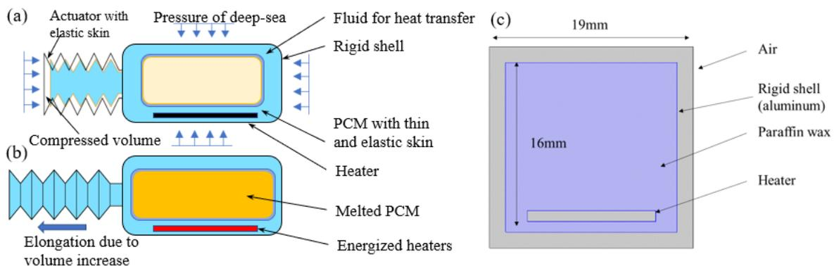
Figure 2. (a) Brief structure of the driver; (b) brief structure of the driver; (c) boundary conditions of the physical model for paraffin phase change cavity. The Z dimension is 150 mm.
