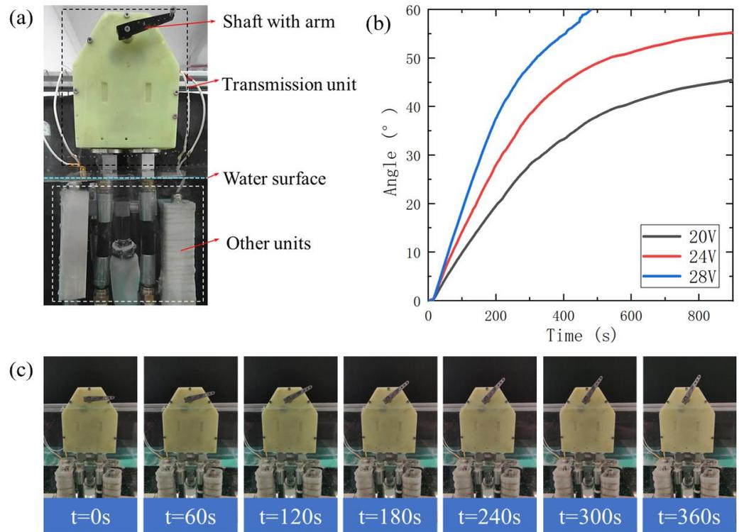
**Figure 8.** (a) The transmission unit and the output shaft are placed on the water to facilitate data collection, the other units are placed underwater, and the phase change storage unit provides power for underwater heating; (b) displacement curve of different heating voltage valves of driving joints underwater; (c) the screenshots at different moments screenshots of underwater experiment.
