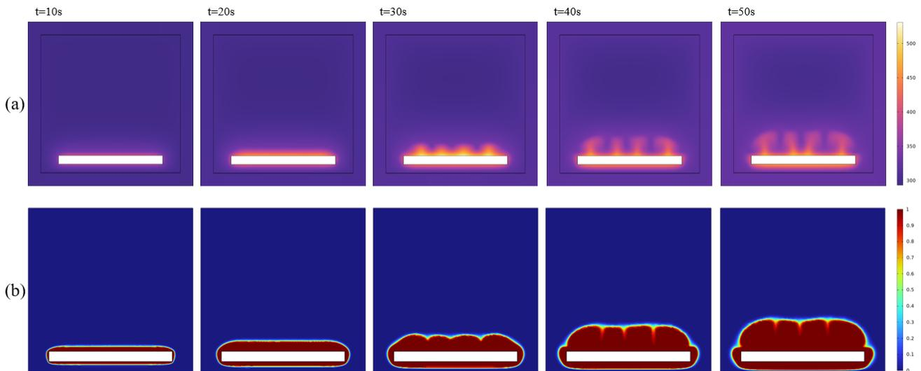
**Figure 3.** (a) Snapshot of the temperature field distribution of the entire actuator within 0–50 s; (b) snapshot of the phase field distribution of the paraffin unit within 0–50 s.
