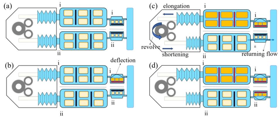
**Figure 6.** (a) Initial state of the joint; (b) preparatory stage, heating valve unit i; (c) operation stage, heating PCM storage unit i; (d) stop operation.
