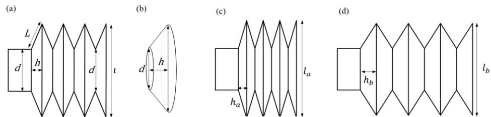
**Figure 4.** (a) Simplified geometric structure of the bellows; (b) individual conical dimensions of the bellows; (c) compressed bellows; (d) extended bellows.
