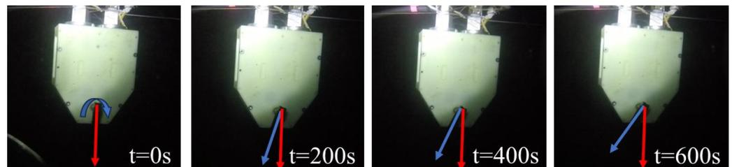
**Figure 11.** Screenshots of output shaft displacement at different moments in the joint drive experiment at room temperature and high pressure (65 MPa). The red arrow in the figure identifies the position of the output arm of the joint at  $t = 0$  s. The blue arrows identify the position of the output arm at different moments of operation.
