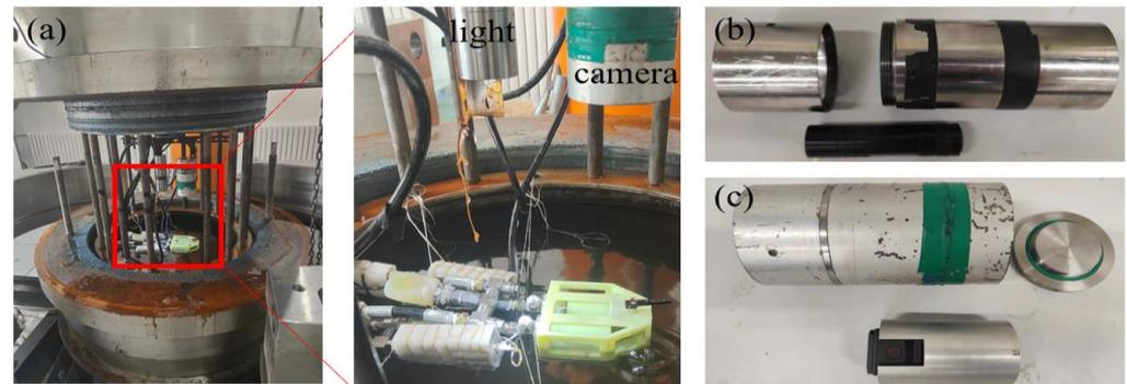
**Figure 10.** (a) High-pressure environment simulation equipment—fix the joint horizontally so that it is suspended and place light and camera on it; (b) lighting equipment and pressure-resistant housing; (c) camera and pressure-resistant housing.
