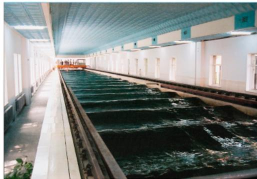
Figure 7. Towing tank.
