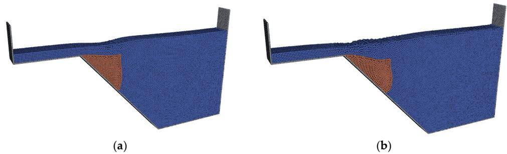
**Figure 2.** Simulated slope configuration and water profile at different moments. (a)  $t = 0.4$  s and (b)  $t = 0.8$  s.
