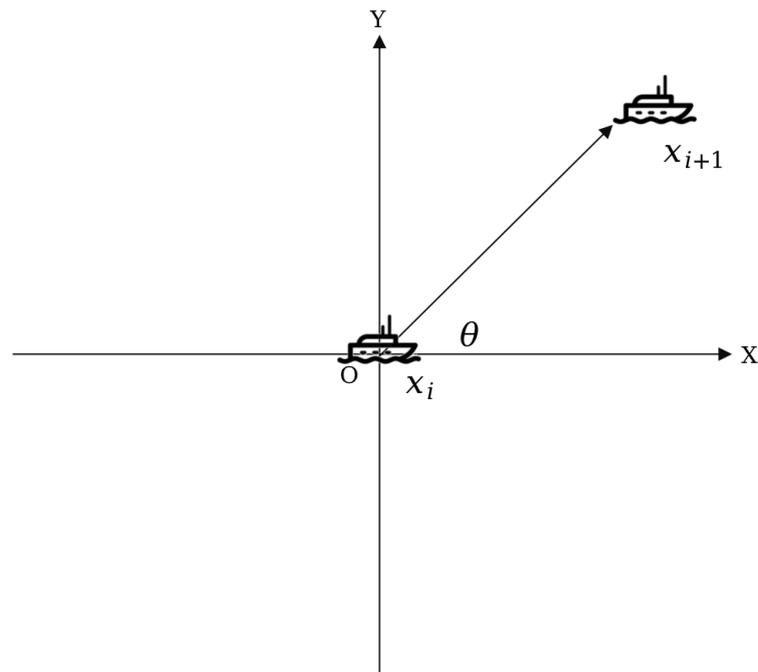
**Figure 1.** A USV motion coordinate system.
