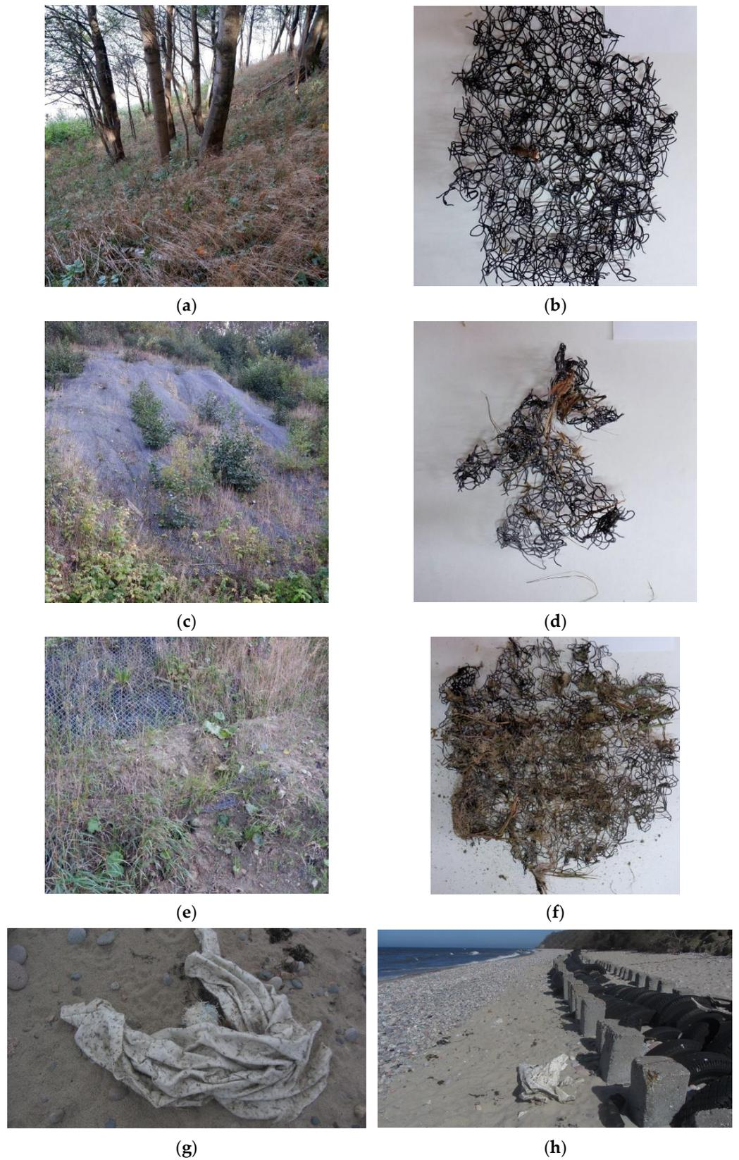
**Figure 4.** Various conditions in which the anti-slide coating is located: the upper, mostly grass-covered (a), and lower (c) (open and with small bushes) parts of the slope or covered by the landslide natural material (e). The samples of geomat taken in these locations (b,d,f). The pieces of geotextile Dornit released from the protection construction were sampled from the beach (g,h).
