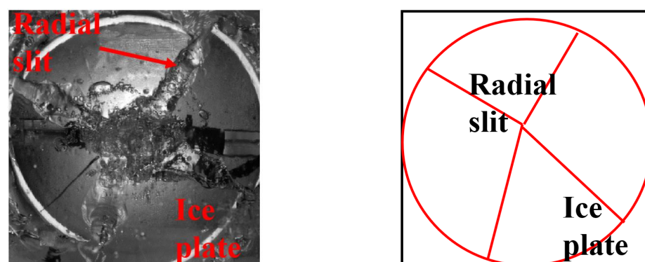
Figure 9. Radial slits pattern when H = 0.53 , T = 0.27 .
